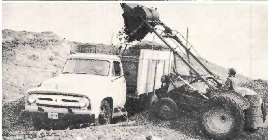
Burs are loaded at cotton gin on truck which has been equipped with special distributing features for spreading compost over farm. Burs will hold a great deal of water—about four times their own weight.
