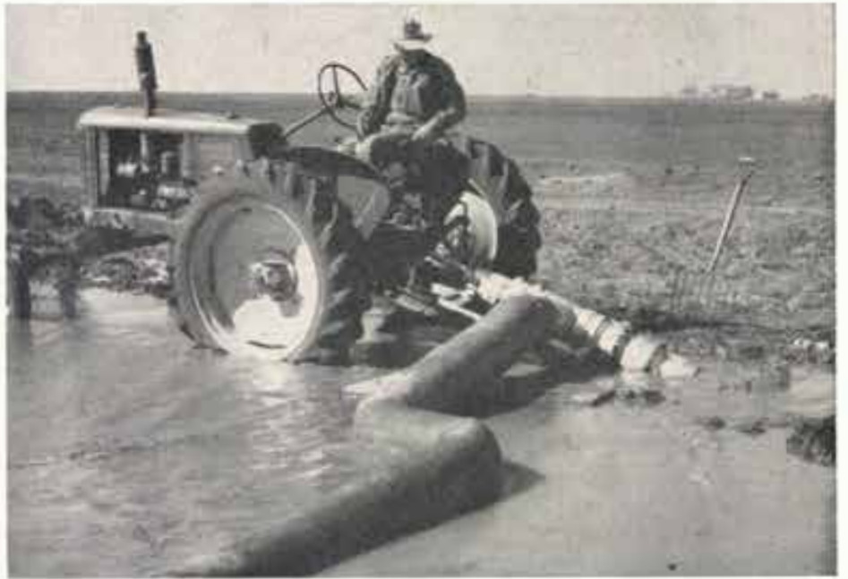
PICKING IT UP —This is a close-up of Charles and his tractor-mounted pump, and shows how waste water is lifted from the end of the field and recirculated through a canvas pipe to the ditch 550 feet away.
