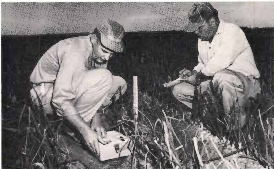
Above, the available moisture present in an onion field is being measured. The moisture available at the depths which blocks are buried registers on the meter dial.
