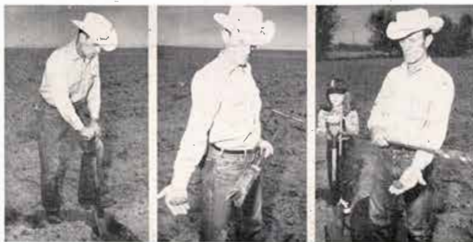
Mr. M. H. Kinard, Lubbock County farmer, demonstrates the use of three simple tools with which soil samples are obtained, (1) the sharpshooter, (2) the core sampler and (3) the soil auger.
