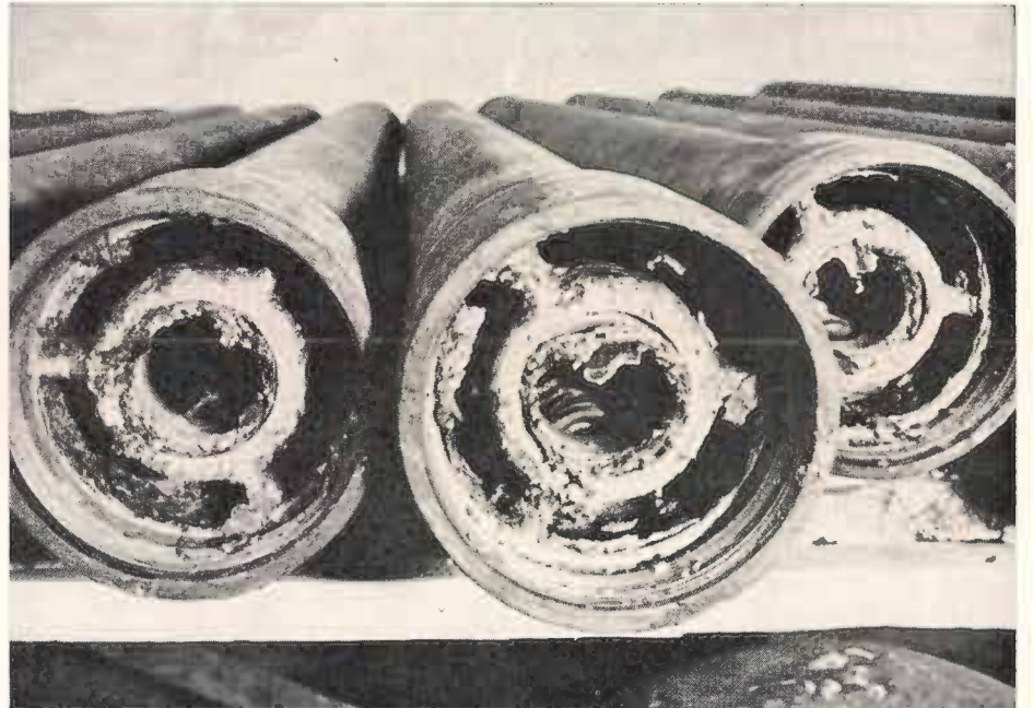
Looking into column pipe laying across the trailer bed the thick mass of algae can be seen covering oil-tube retainers. Algae was present on the outside of column pipe only from the static water line downward.
