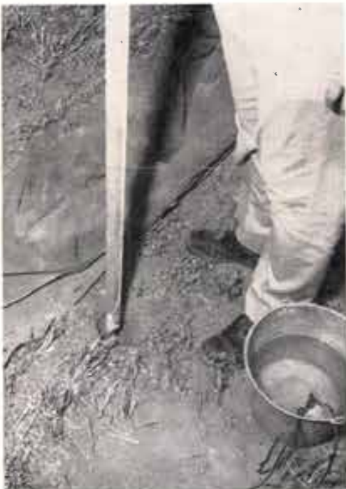
Block is placed at measured depth below surface. Wires from electrodes lead to the surface. (4) Shallowest
