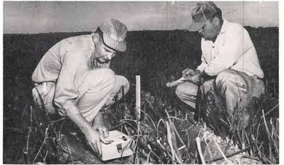
Available moisture present in the root zone of the Floyd County onion field is being checked by District field representatives. They are using a moisture meter to read percentages of available moisture in blocks of gypsum buried beneath the surface.
