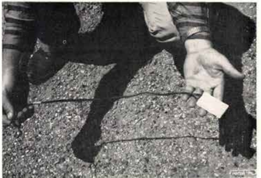
Gypsum blocks that contain small electrodes are buried at various soil depths throughout field. Colored wires lead to the surface from imbedded electrodes. Each color represents a certain depth at which block is buried below surface. Readings are taken by attaching meter to electrode wires.
