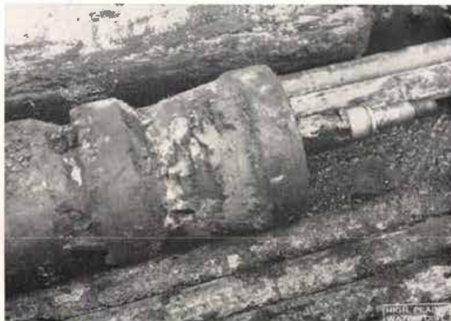
The dark greasy-like algae and bacteria growth which covers the pump bowl-assembly shown above can clog well casing perforations and even the pores of the water-bearing formation.
