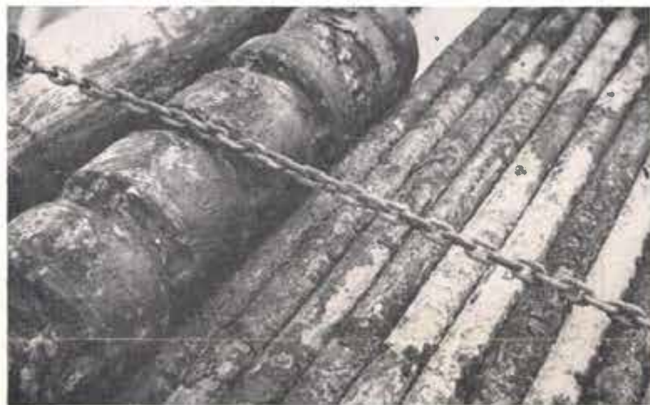
Above is shown a pump bowl-assembly on the left and oil tubing at the right which has just been pulled from an irrigation well. The encrustation visible on these pump parts is Blue-Green Algae accompanied by Iron and Sulphur Bacteria.
