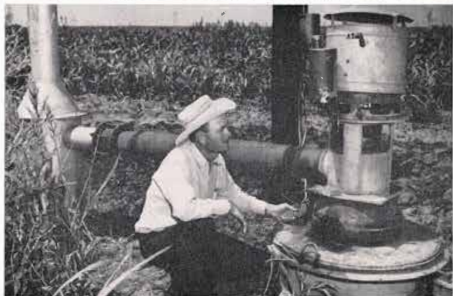
Mr. Belt checks the automatic float control that turns his recirculating pump on and off. When the sump fills with "tailwater" the pump starts automatically, returning the water to the high side of the field where it can again be used.
