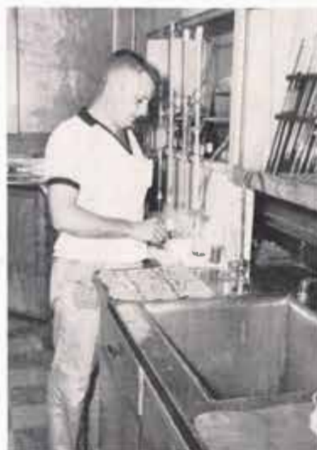
Water quality tests are continually run in the station's laboratory. Here Dale Hanna, station laboratory operator, prepares to check both the boiler water and the cooling-tower water.
