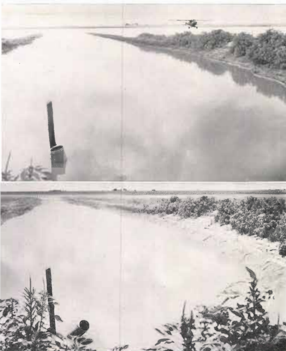
Picture at top shows airplane spraying the Weaver lake with a liquid flocculating chemical. The bottom picture was taken 4 days later after the lake water, except a small quantity that remained in the pit at the recharge well intake, was drained by gravity into the underground formations.
