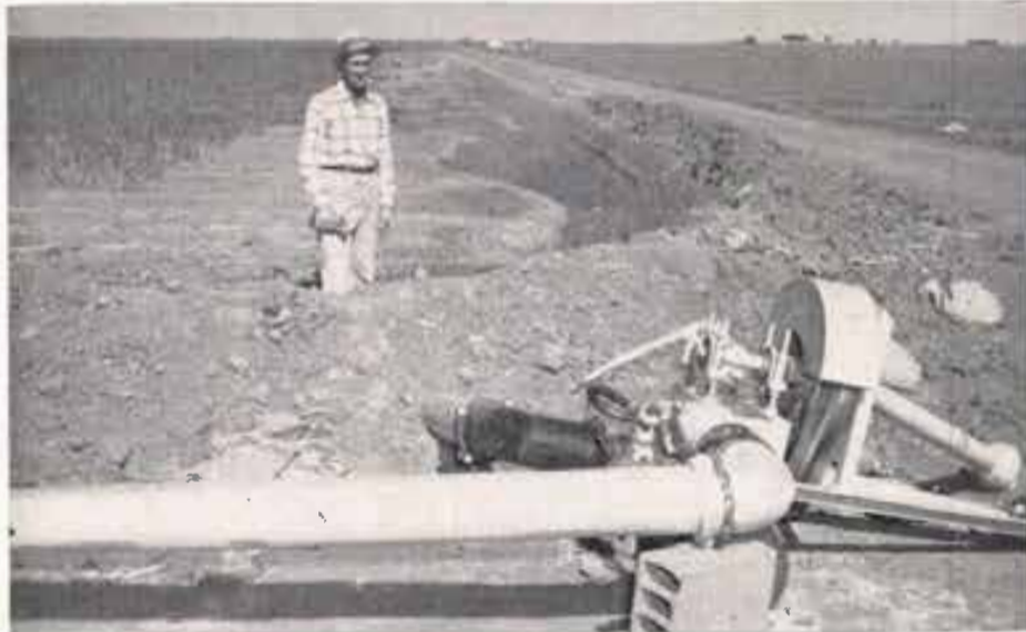
M. B. Newton inspects the small "tailwater" pit at the low corner of the farm. After irrigation water reaches the end of the field, it comes to this corner where it is picked up by the centrifugal pump shown in the foreground and sent through the 6-inch aluminum pipe to an open ditch one-fourth mile up the field. There it commences its journey back down the crop rows.
