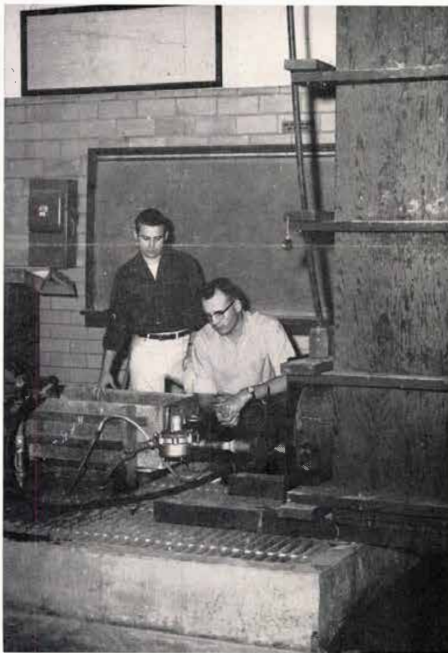
D. B. Underwood, left, and Delbert Smith, Texas Tech students watch as meter records quantity of water passing through gravel filter enclosed in box at right. Recharging underground sands with raw lake water presents problems of clogging the formations. The model filter system attempts to simulate field conditions and extract suspended particles that cause clogging.
