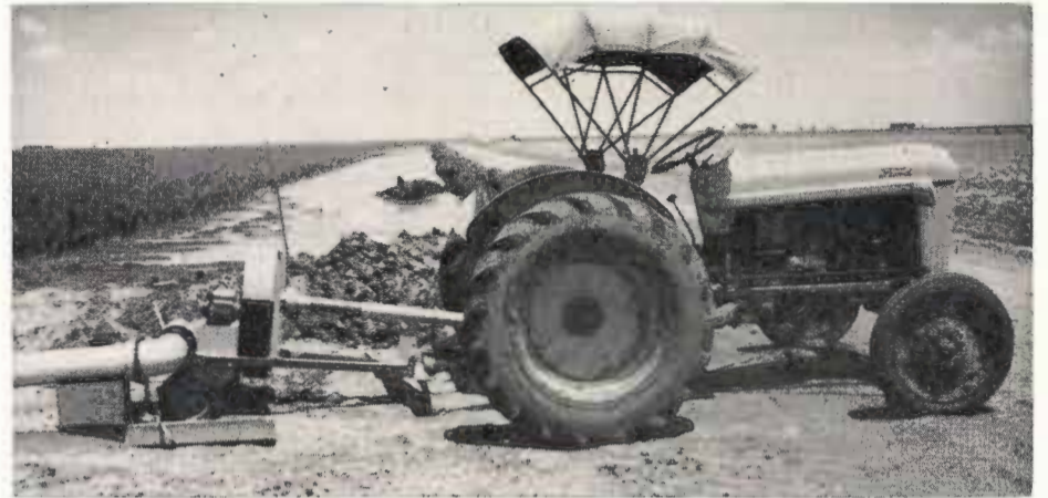
The general-purpose farm tractor shown furnishes power for the 3-inch centrifugal pump. The small pump is completely portable and can be moved anywhere on the Newton's farmland.
