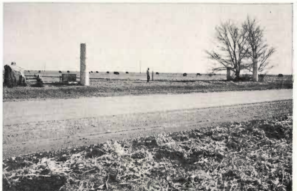
One of four irrigation wells on the Shurbet farm is shown above at left. Only a short distance from this production well is an observation well, right, in which the water level is measured. An automatic recorder is installed in the well. It continually records fluctuations in the underground water level. This record will be important in substantiating depletion.
