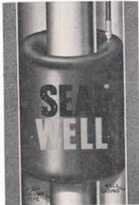
Figure 1 An inflatable "doughnut" seal was installed between the pump's column pipe and the well casing to prevent air from entering the well and becoming entrapped in the water-bearing formation.
