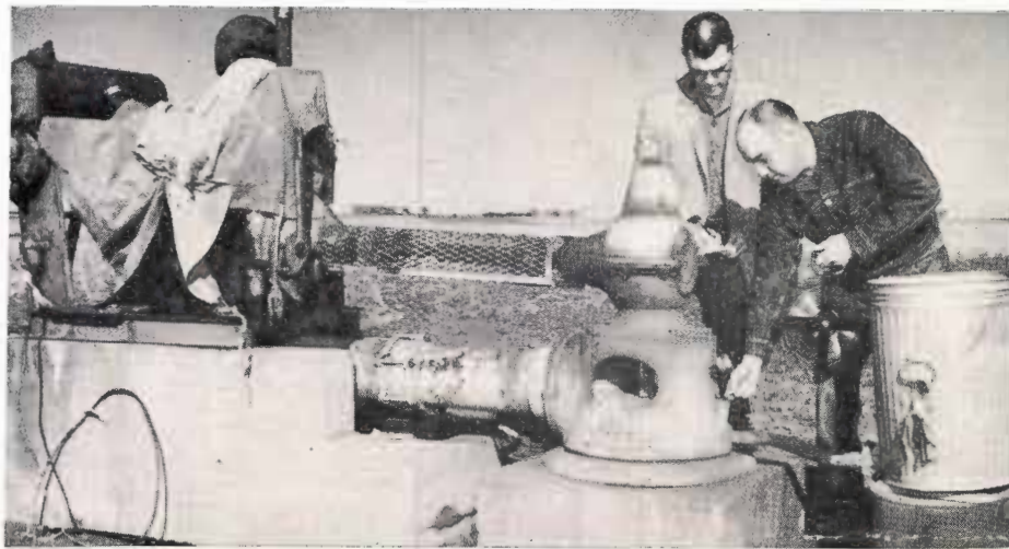
Don Reddell prepares to record the depth to the water level below land surface in this observation well. Y. F. Snodgrass unreels a steel tape into the well to make the measurement. Both men are High Plains Water District staff members. Water levels in hundreds of southern High Plains observation wells are measured annually.
