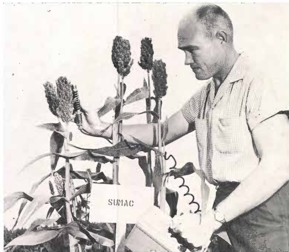
More basic research and new approaches to research are needed in order to continue progress in agriculture. This photo shows how a geiger counter is used to study root systems in plants by following translocation of radioactive phosphorus placed in the soil. This is part of a research project on root systems of plants being undertaken at Texas Tech in cooperation with the Texas Agricultural Experiment Station.
