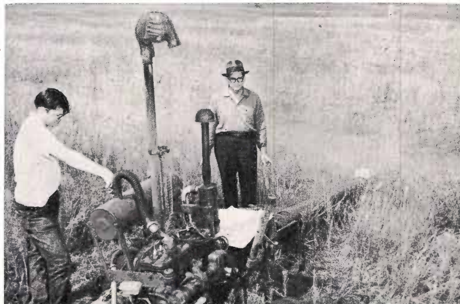
Donald Reddell, left, and W. L. Broadhurst, High Plains Water District staff members, are shown as they start the engine of a pump to empty a playa lake of water. The lake is one of several being studied by the Water District and the Lubbock City-County Health Unit. It will be modified, by removing dirt from the bottom, to concentrate the water in a smaller area.
