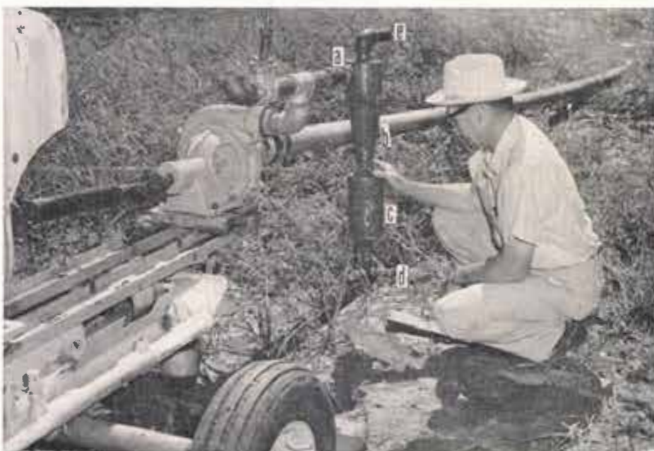
W. L. Broadhurst, Chief Hydrologist for the High Plains Water District, is shown above as he inspects an instrument designed to remove suspended particles from playa lake water prior to using it for recharging the ground-water reservoir. Various parts of the instrument, designated by letters, are referred to in the story at right.
