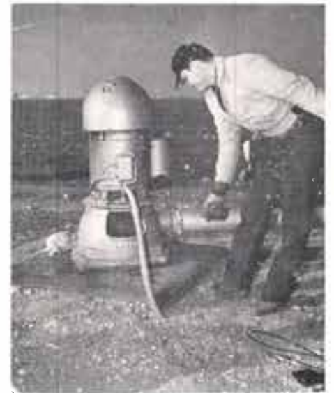
Above are shown two High Plains Water District staff members, Wayne Wyatt, at left, and Don Reddell, as they make measurements of the static water level in two of the hundreds of observation wells measured each year in the Water District. The annual measurements have been completed for 1962 and "The Cross Section" will publish them in the immediate future.
