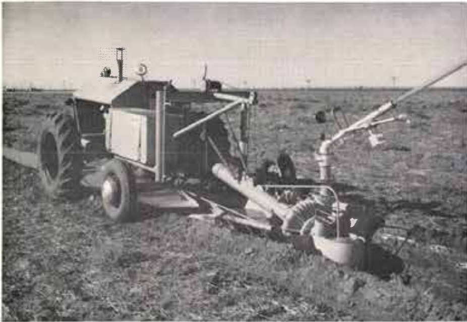
Above is shown the "Waterdog" irrigator as it pumps irrigation water from an ordinary open ditch to the young wheat crop. Harold House, a Clovis, N. M. farmer, said the sprinkler machine solved his irrigation "tailwater" problems. He says that with the machine, he can uniformly distribute the required amount of water over his land.
