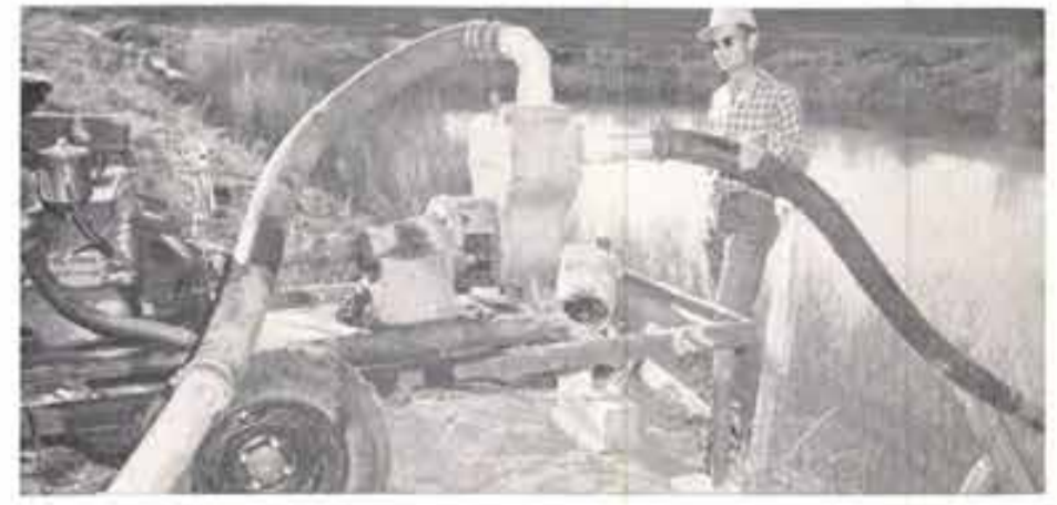
Riethmayer inspects the 4-inch self-priming centrifugal pump used in his "tailwater" re-circulation systems. Like the other, this pump can be used at any of the three collection pits. Only two of the three pits are ever used simultaneously because only two-thirds of the total acreage is cropped simultaneously. The remaining land is fallowed.
