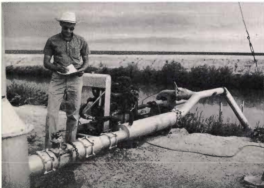
Dick Godwin, Deaf Smith County irrigator, is shown as he records the number of gallons of "tailwater" pumped back to cropland through his re-circulation system. The High Plains Water District is furnishing, on a temporary basis, the flow-meter being used by Godwin to calculate the quantity of water.
