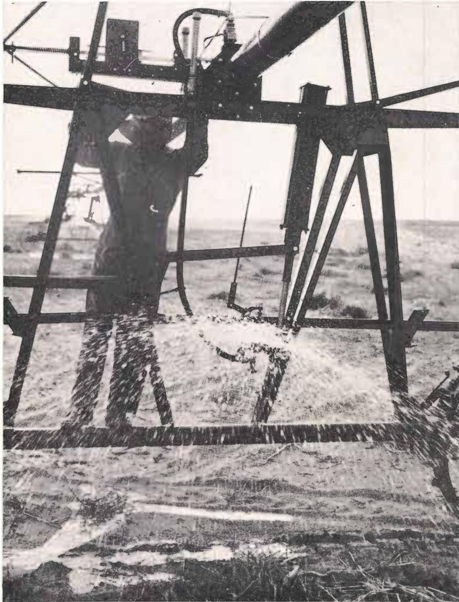
When the cylinder fills with water a relief valve is actuated that empties it onto the soil surface, and as this occurs, the horizontal bar engages with the next set of wheel lugs.
