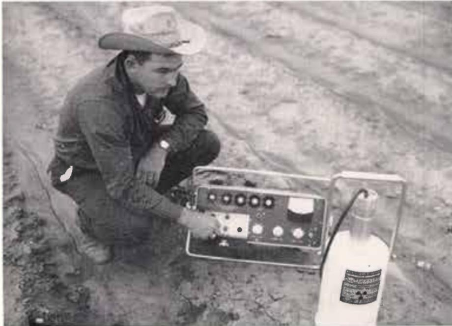
J. S. Newman, Irrigation Specialist at the Experiment Substation near Lubbock, is shown as he manipulates a neutron tube. The device has recently been added to the station's equipment inventory. Its function is to measure moisture in the soil by using a radioactive material. The neutron tube will be used in the station's irrigation and water research work.
