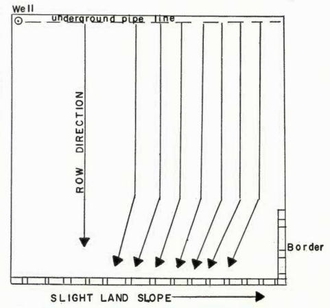
If you have land that slopes in two directions, contoured rows can save water. Tailwater can be conserved by watering from north to south with rows angling across from northeast to southwest. The angled rows at the end of the field should be almost level from one end to the other.
