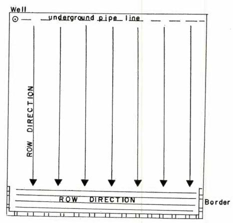
One water conservation practice is to drill or plant a crop parallel to the ends of the normal row direction. This practice is especially efficient for land with a general slope in one direction.
