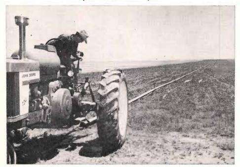
Shofner pointed out that one of the more important steps to remember in moving the tow-move lateral lines is to allow complete drainage of water from the line before movement is commenced. Damage to the couplings may result unless this basic rule is followed. Each 30-foot length of lateral pipe has its own automatic draining mechanism to facilitate this phase.
