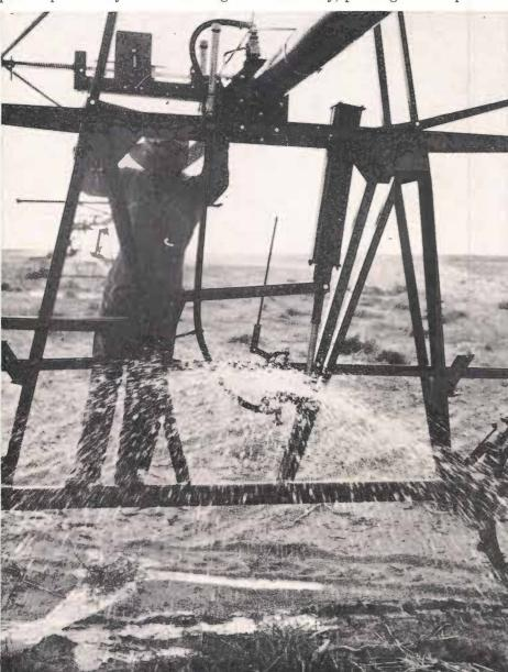
When the cylinder fills with water a relief valve is actuated that empties it onto the soil surface, and as this occurs, the horizontal bar engages with the next set of wheel lugs.
