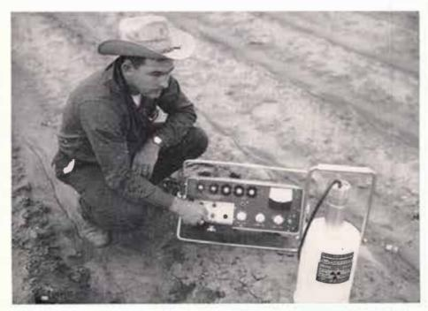
J. S. Newman, Irrigation Specialist at the Experiment Substation near Lubbock, is shown as he manipulates a neutron tube. The device has recently been added to the station's equipment inventory. Its function is to measure moisture in the soil by using a radioactive material. The neutron tube will be used in the station's irrigation and water research work.
