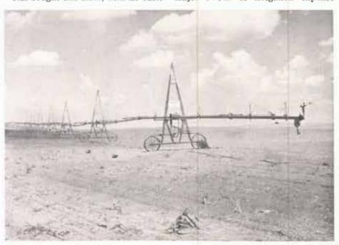
The self-propelled sprinkler system moves in a straight line around a pivot point at the center of the square-shaped farm.
