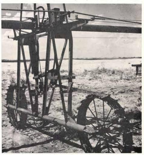
Note manner in which the horizontal bar engages with the wheel lugs when the cylinder is emptied. It is now prepared to slowly move the tower, and thus the pipeline, as the cylinder fills with water.
