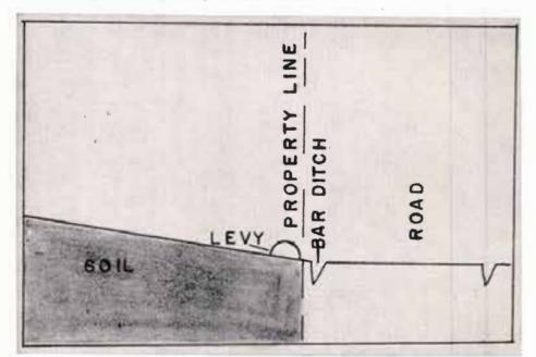
Sometimes building border and then plowing it down can present a problem. An answer to this problem is to get a maintainer to roll a broad border that you can plow over but will hold the tailwater in the field. This illustration shows the levy in an extremity, it should be more sloping to facilitate plowing over.
