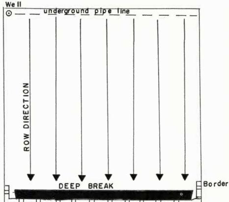
Deep breaking across the lower end of a field with a general slope in one direction can stop the flow of tailwater. In using this practice it is necessary to construct a border beyond the deep breaking to prevent the tailwater from channeling.
