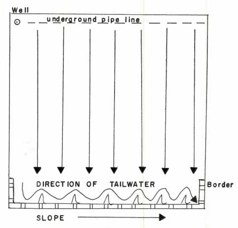
On a farm where land has a two direction slope a border can be constructed around the lower end of the farm. At approximately two foot intervals a diverter can be run toward the rows. this will slow down and back-up tailwater in a manner as to soak the land before the water moves to the next section.
