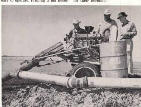
The certrifugal pump that is manufactured by KMP Pump Co. of Earth will pump at almost any angle. This easy to operate unit which the Whites have is fueled by a 55 gallon gasoline drum and uses about one and one-half gallons of gasoline per hour of pumping time.
