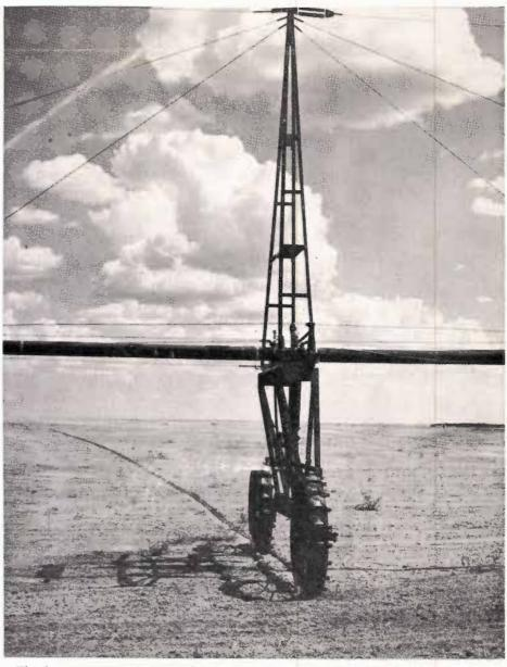
The lugs on each wheel play a two-fold role. First, they prevent slippage, and second, they are used in transmitting power from the water cylinder to the wheels. The wheels track in the same path each revolution of the system.
