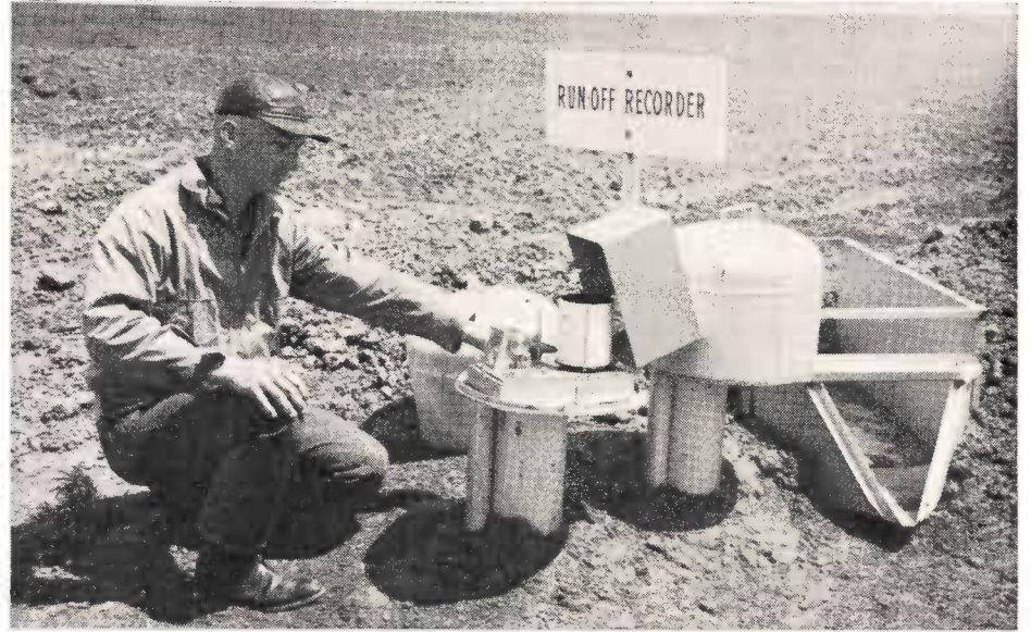
James Zetzsche, agricultural engineer at the Research Center points out the recording device that is being used to record the amount of water passing through the recording flume. The device also records the time that the water passes through, giving researchers valuable data on runoff water.
