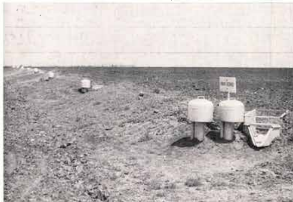
Above is a line-up of the run-off recording devices that are being used to record the amount of water lost from the fifteen plots of land that are under study at the Research Center.
