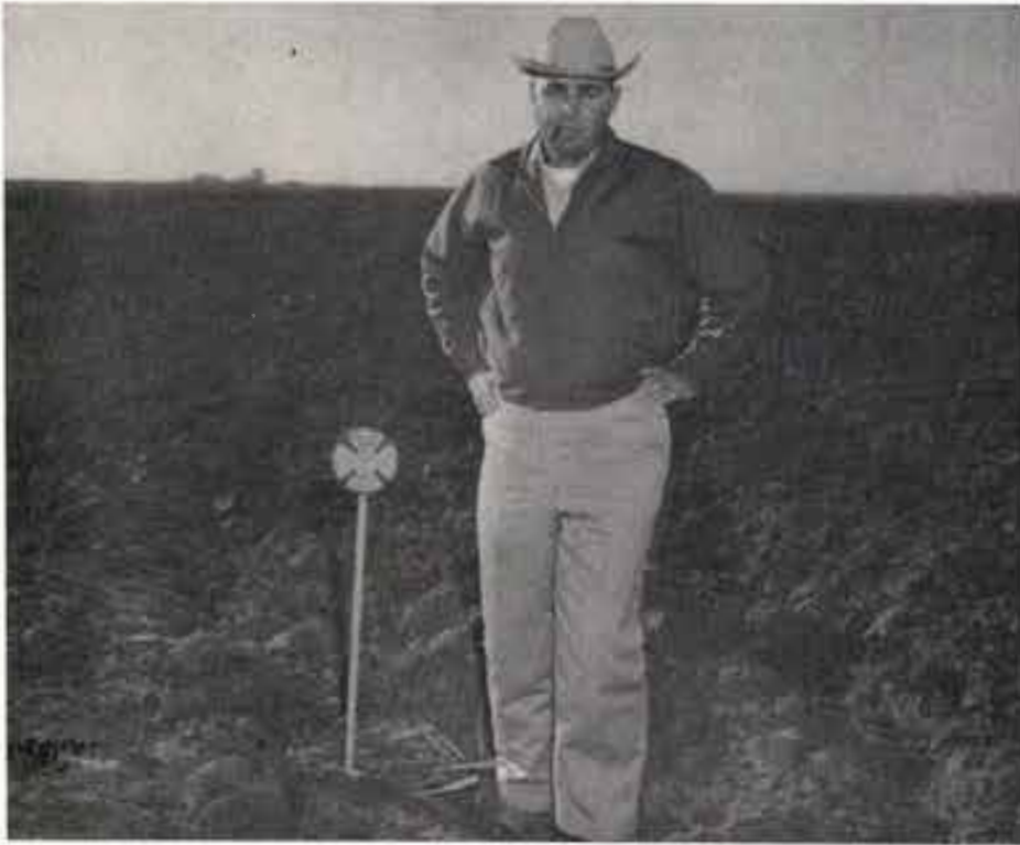
The Break-Over Marker, invented by Don McInturff, allows the tractor operator to break the soil very close to the valve. The operator does not have to dismount but can drive his tractor over the Alfalfa Valve protector.
