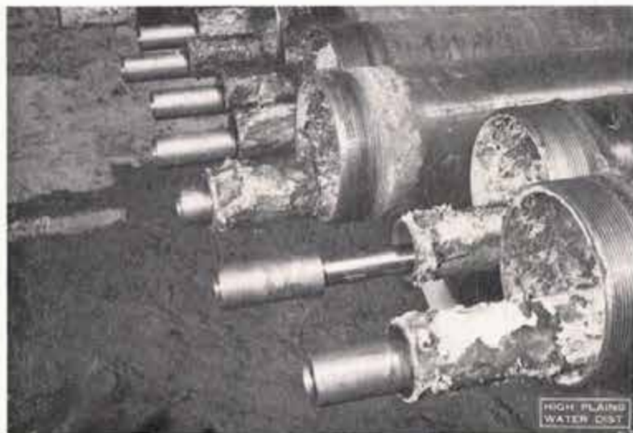
Proper chemical treatment will remove, or better, will prevent "build-ups" like this on pumping equipment.
