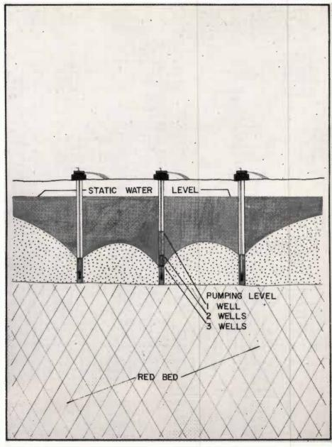
Above sketch shows effects of wells on pumping level. Note difference in one well and three wells.
