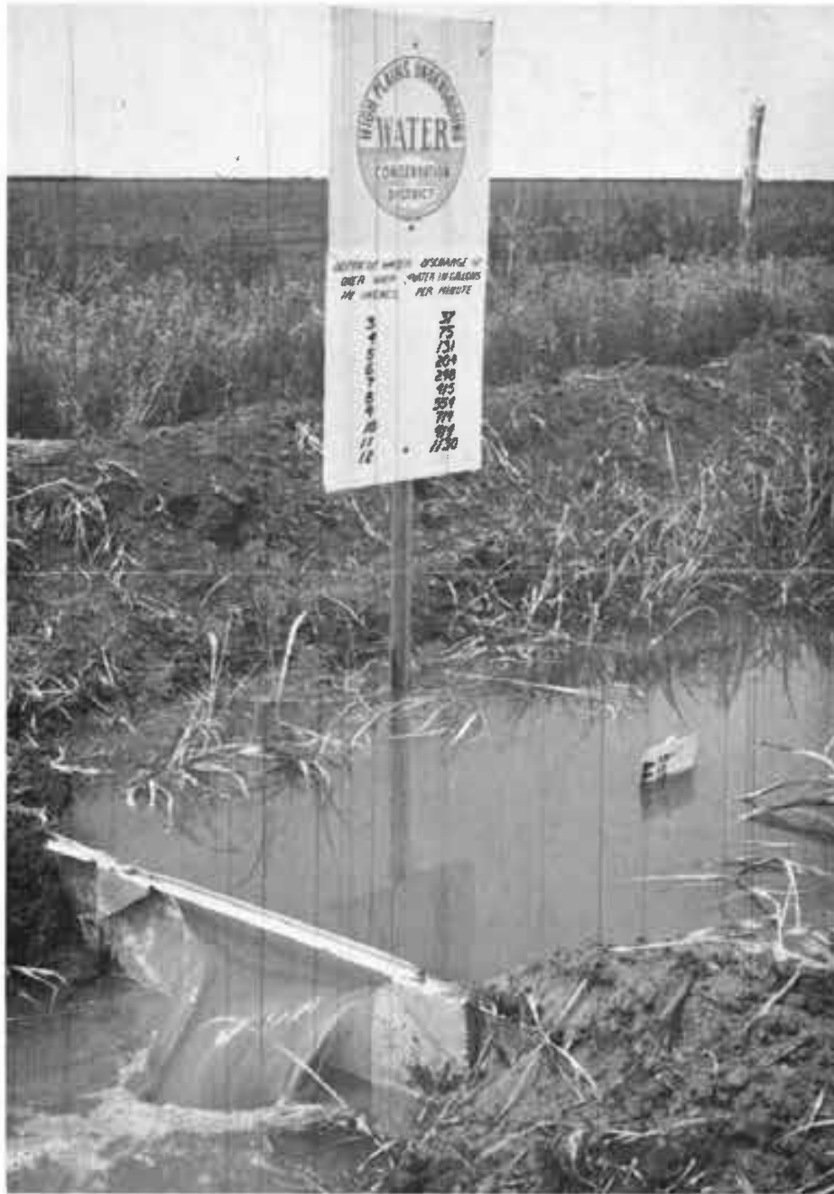
A weir with water being measured. Read the depth of the water in inches in the ditch and apply it to the large sign.
