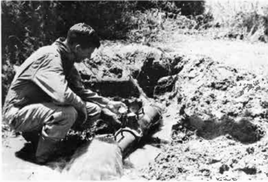
Albert Sechrist is shown above using a turbine flow meter to measure the amount of water pumped by an irrigation well during the Irrigation Cost and Efficiency Research.
