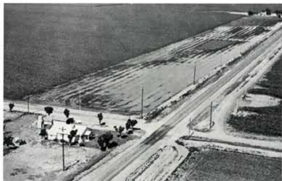
A border is never the answer to the need for a permanent tailwater return system. This photograph shows a border that is retaining the tailwater from the irrigated cornfield, on the farmer's land, and is, therefore, in technical compliance with the District's waste abatement policies. However, the loss of groundwater through percolation and evaporation is excessive. The magnitude of this tailwater runoff, and the physical conditions on this field, are readily adaptable to groundwater conservation through a permanent tailwater return system. The land recovered for additional crop or cattle production would more than defray the costs of a tailwater return system. This is the only condition of gross flooding of land by tailwater runoff observed during a recent aerial tour of the northeastern part of the District.
