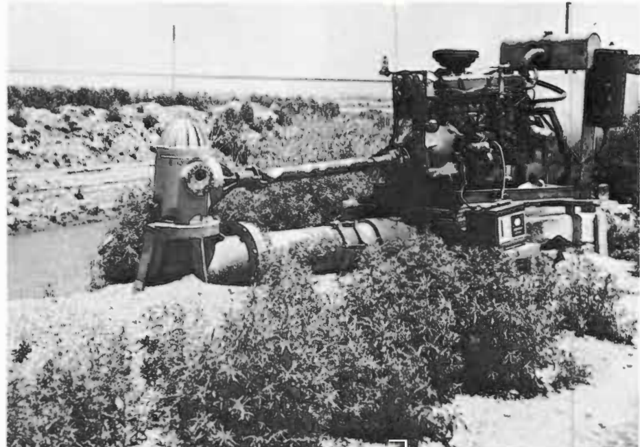
The new tailwater return system is powered by a six-cylinder butane engine. Reznik says this engine is good in that it does not freeze up in the winter. He waters stock during the winter months with tailwater from this pit.
