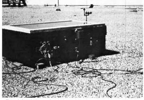
Pictured above is the experimental heater designed by the Texas A&M researchers for the specific purpose of correlating operating variables in the testing of their concept of space heating.
