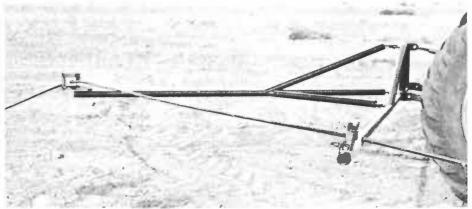
A method for transporting a drip irrigation emitter hose in a field of cotton is a second technique being advanced. A simple attachment behind a tractor enables the hose to be moved quickly from one row to another without stopping the well pump.
