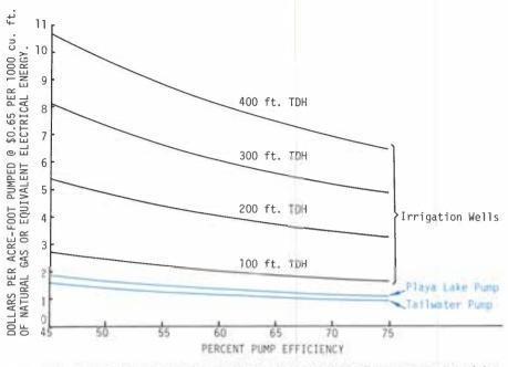
Figure 1. Representative energy costs per acre-foot for tailwater and playa lake pumps and for irrigation wells with different pumping heads.
