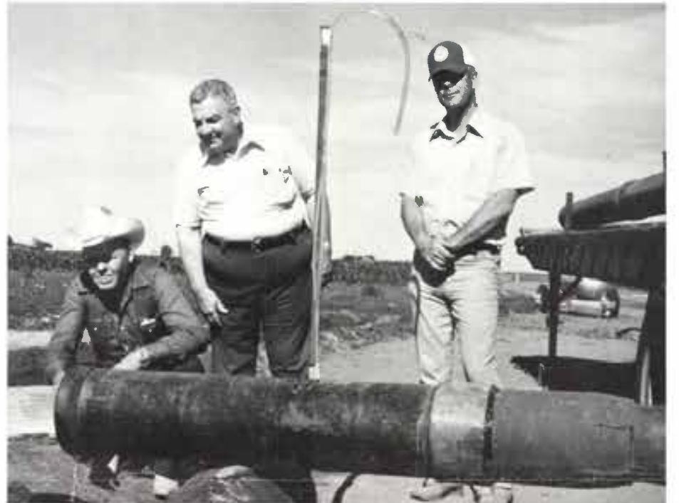
Don Marble and Solon Clements, President and Member of the Board of Directors of the High Plains Research Foundation respectively, and Dr. Bill Lyle, observe the (orifice plate) measurement of the pumping rate (1300 gallons per minute) of the new irrigation well on the Texas A & M University Agricultural Research and Extension Service Halfway (Hale County) Station.
