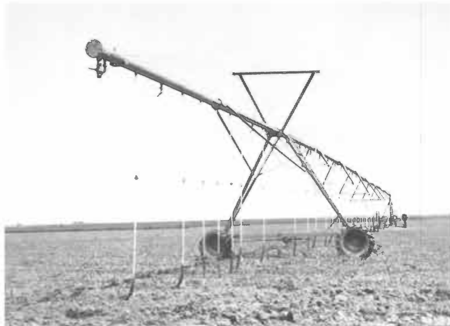
This center pivot irrigation system, on the Texas A & M University Halfway Research Station has been modified by Dr. Otto Wilke, to apply irrigation water at the land surface, curtailing the evaporation and temperature losses common to sprinkler irrigation. This system would be readily adaptable to furrow diked fields. This system is automatically controlled by moisture sensors.
