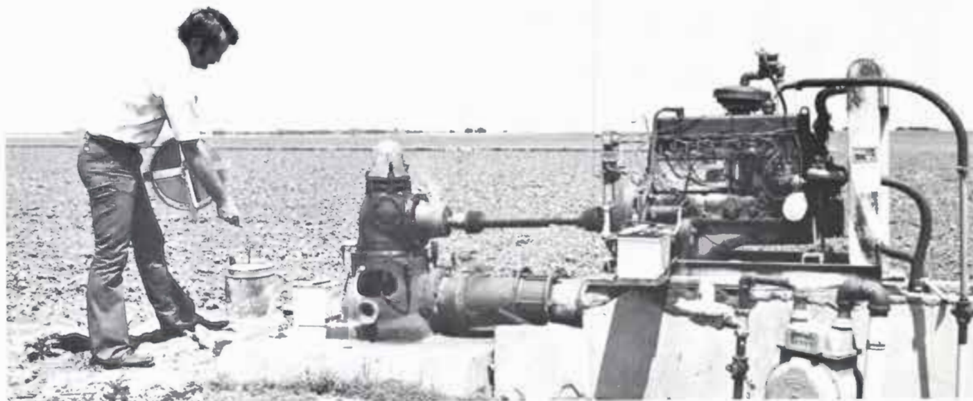
District Field Representative Butch Bates measures the depth to water in an observation well by inserting a steel tape into the well. Each January, the District conducts such measurements in more than 800 wells lying within the boundaries of
