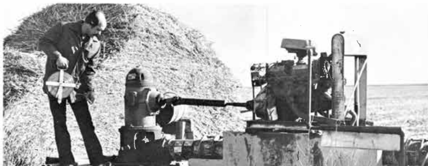
District Field Representative Oscar Riemer measures the depth to water in an observation well by inserting a steel tape into the well. Each January, the District conducts such measurements in more than 800 wells lying within the boundaries of the District
