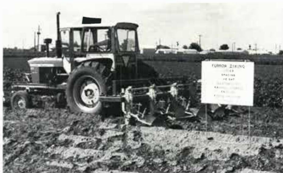
The Texas Agriculture Experiment Station at Lubbock observed its 68th Annual Field Day on September 13th. Pictured is the basin tillage tool designed to form small mounds of soil at intervals along the furrow and in effect build small dams to prevent rainfall runoff.
