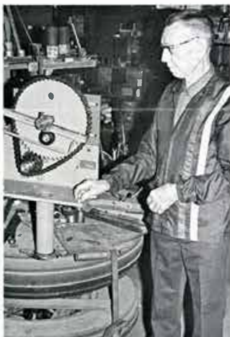
"Mr. Gus" stands by the patented windmill drive from one of the new windmills produced at his company. The chain and sprocket drive on these windmills eliminates the need for a gear box of any kind, thus keeping down possible future repair costs.
