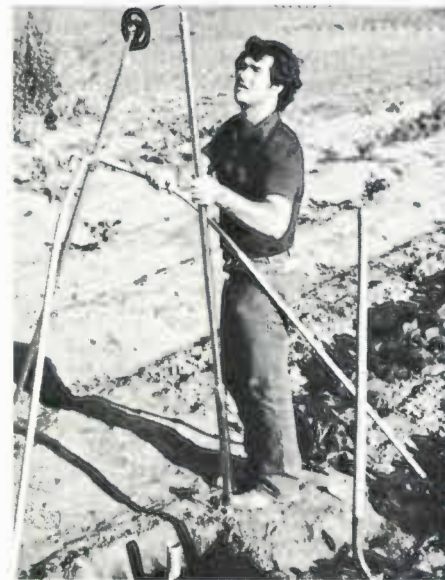
HOOKIN' IT , Dwight Adams aligns the probe over the tripod above the access tube.
