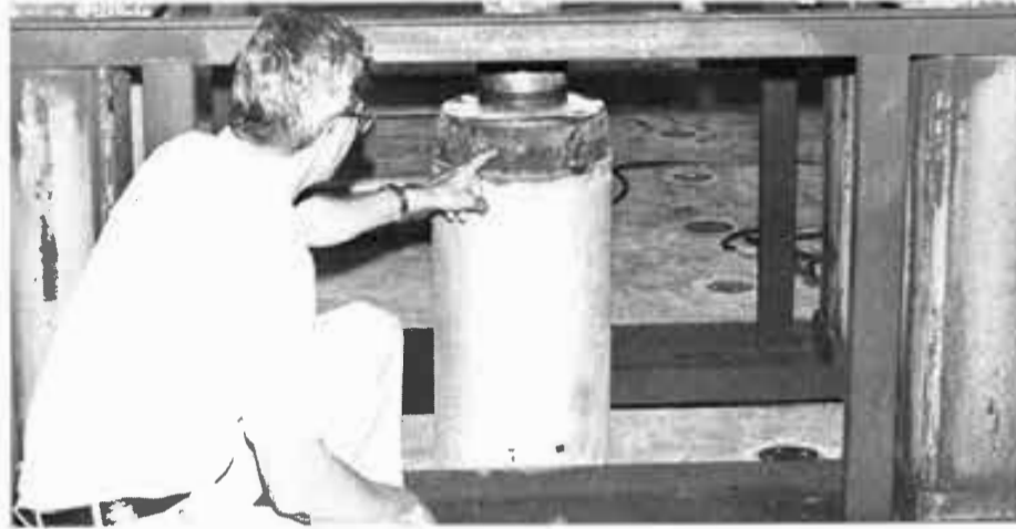
IN THE LAB Bill Claborn points out the tire assembly section of the pneumatic bag snuggled into a model well casing. In the four corners stand hydraulic jacks in a steel frame. The unit is capable of lifting 500 thousand pounds.
