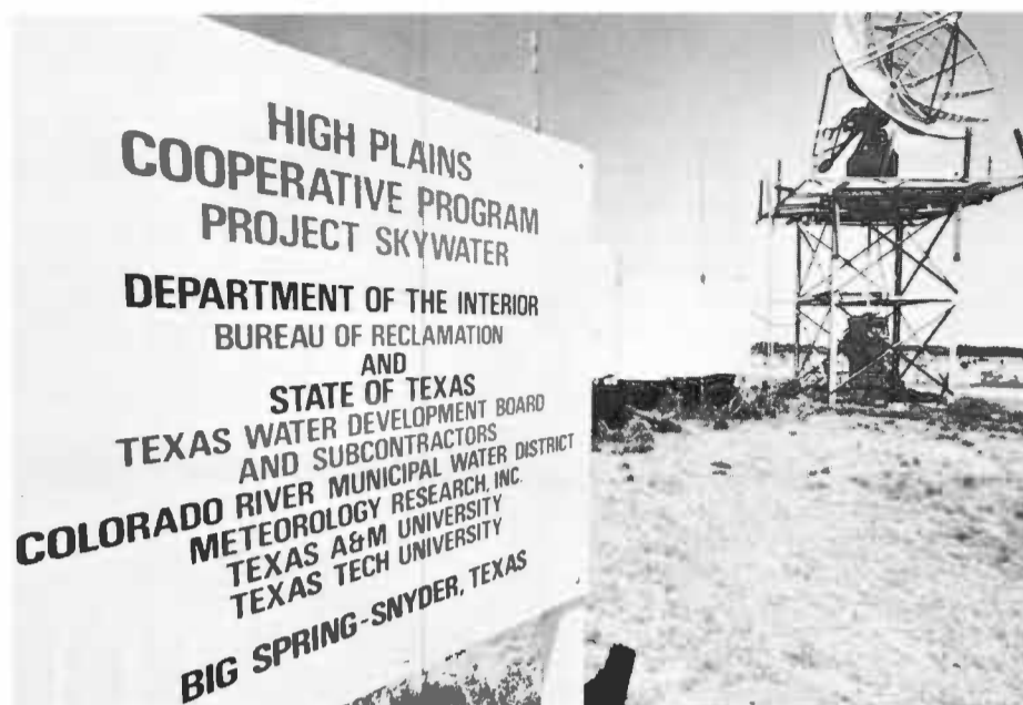
Radar, located near Snyder, Texas, records the location, size, and motion of clouds over the HIPLEX area and provides estimates of the rainfall.
