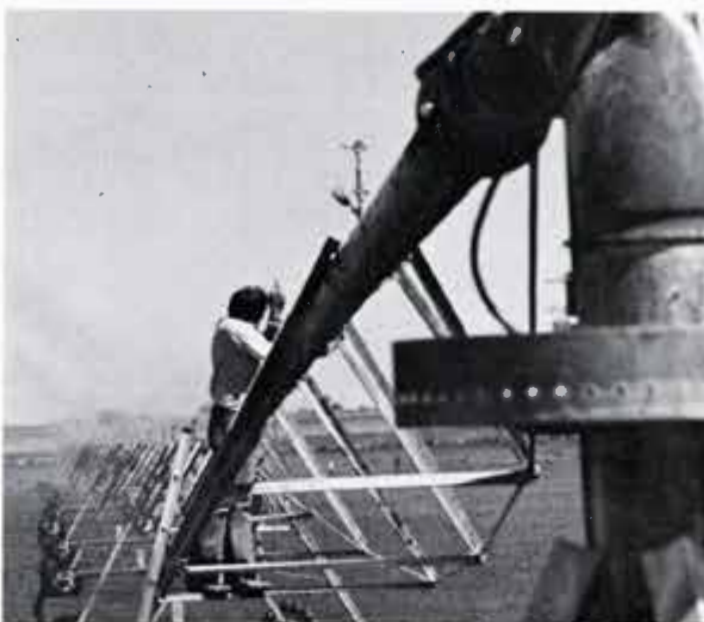
RIDING HIGH atop a center pivot system Bob gets a water reading before a hose is attached to the sprinkler head. Water is drained into a five gallon bucket to determine the gallons per minute discharged by a single nozzle.
