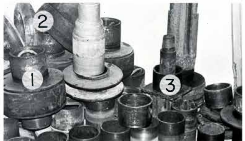
FOR SALE: Thirty slightly used go-cart tires and pipe fittings. 1. Typical assembled gripping device of tire, placement washer and connecting hose. 2. Stock item go-cart tires and tubes used in gripping assembly. 3. Drill pipe used inside for additional strength.
