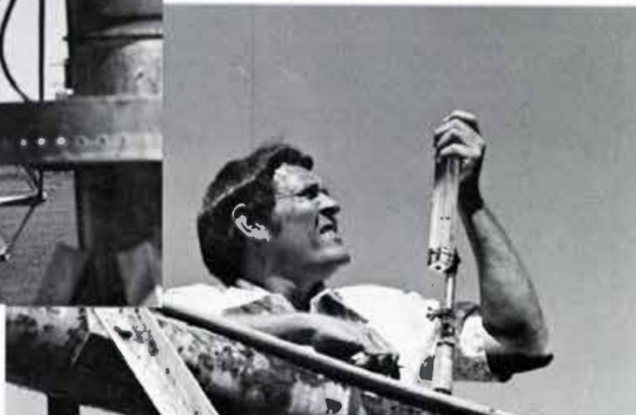
SPEED READER , Bob Arhelger of the Soil Conservation Service in Lubbock checks the water velocity through a center pivot system during workshop tests. The speed at which water is moving through the system helps determine the gallons per minute being discharged by the system's nozzles.
