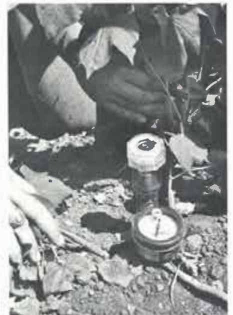
TENSION MOUNTS as the tensiometer reading reflects less water available to the plant.
