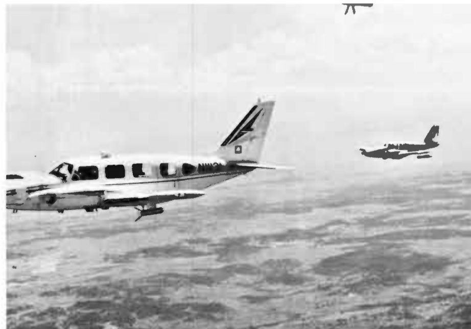
Instrumented aircraft fly in and around convective clouds to study their characteristics and observe the effects of seeding.
