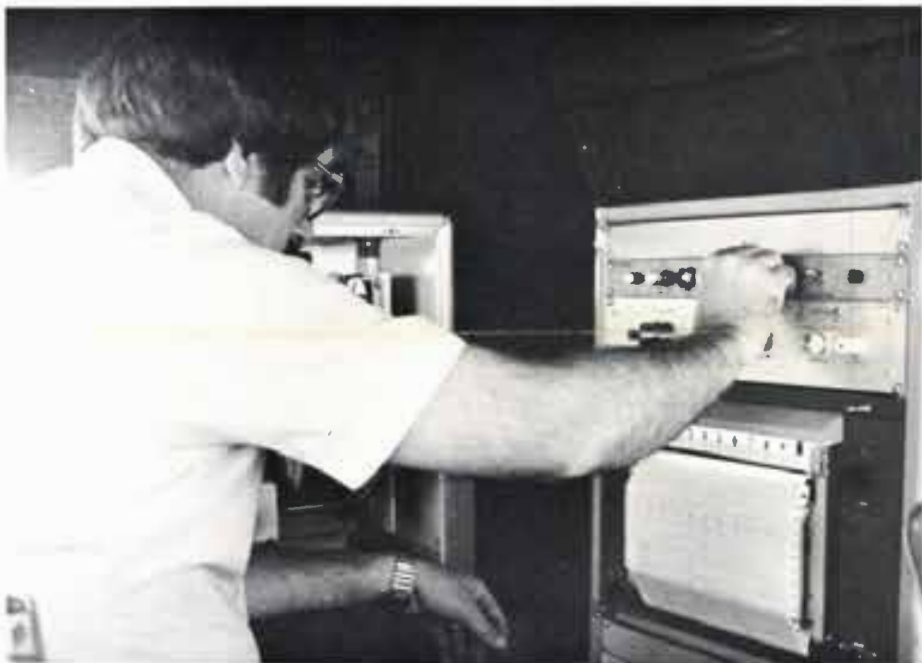
PLOTTING ALONG , Ken Carver calibrates the geo-logger to record soil moisture levels from the full depth of the probe hole.
