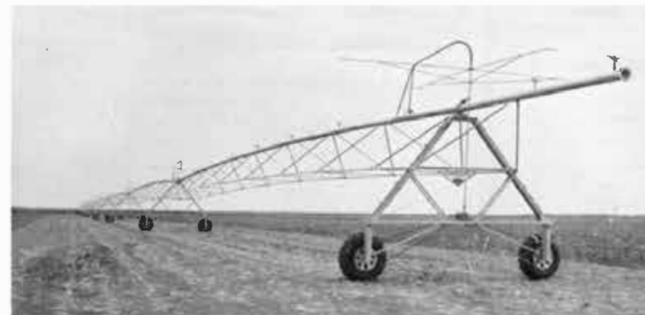
The electric drive center pivot with high pressure impact nozzles were very popular in the 60's and 70's.
