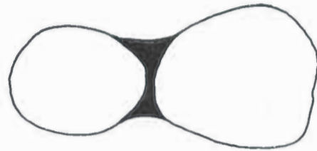
CAPILLARY WATER in the unsaturated zone held by tension.
