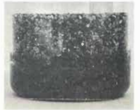
TRAPPED WATER remains in the sand and gravel above the free water table.
