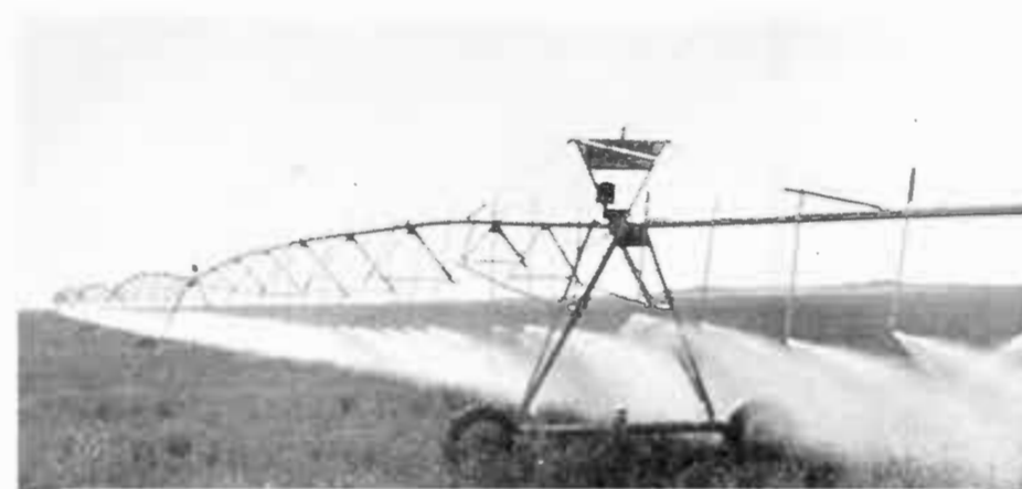
Low pressure systems were developed to cut energy and evaporation losses.
