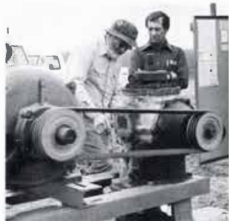
MEASURING DRAWDOWN, Raymond Benham tested Bob's well three times.
