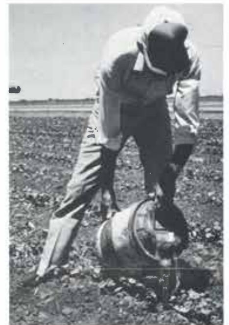
TENSIOMETERS installed in a cotton field measure soil moisture and help signal when to irrigate.
