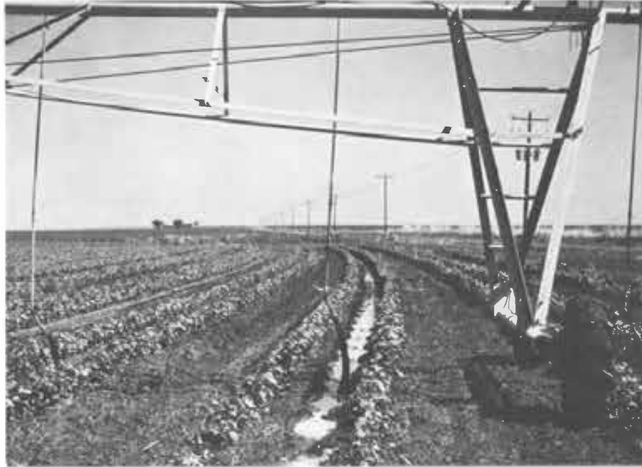
HIGHLY EFFICIENT , very low pressure sprinkler systems circle the crop and lay water right down into the furrow where mini-dams prevent the water from running.
