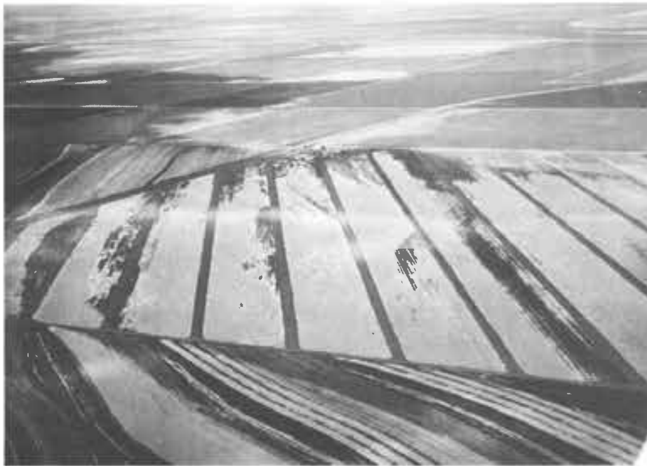
PARALLEL TERRACES catch and hold rainfall in the field to prevent runoff and soil erosion.
