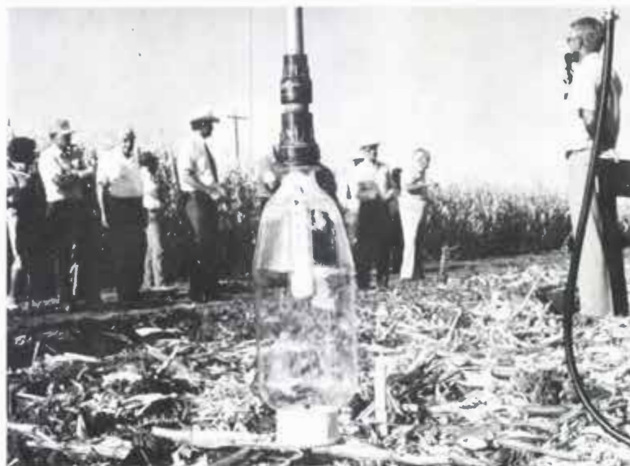
ON THE ROAD —In Dumas, Bill Lyle, TAES Agriculture Engineer at Lubbock, explains the design of an experimental dropline nozzle which reduces soil erosion in the furrow under a low pressure sprinkler.
