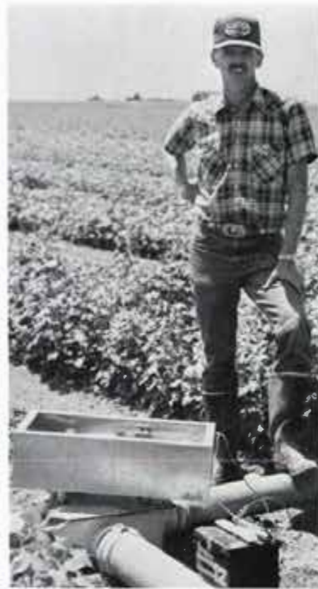
A NEW CONTRAPTION —Roger Kitten explains what he likes about surging. The battery powered timer controls when the gear switches water from a set on one side of the valve to a set on the other. The valve openings are sealed by a moveable rubber disk. (Valve manufactured by Aluminum Metal Products, control box by Lubbock Electric.)
