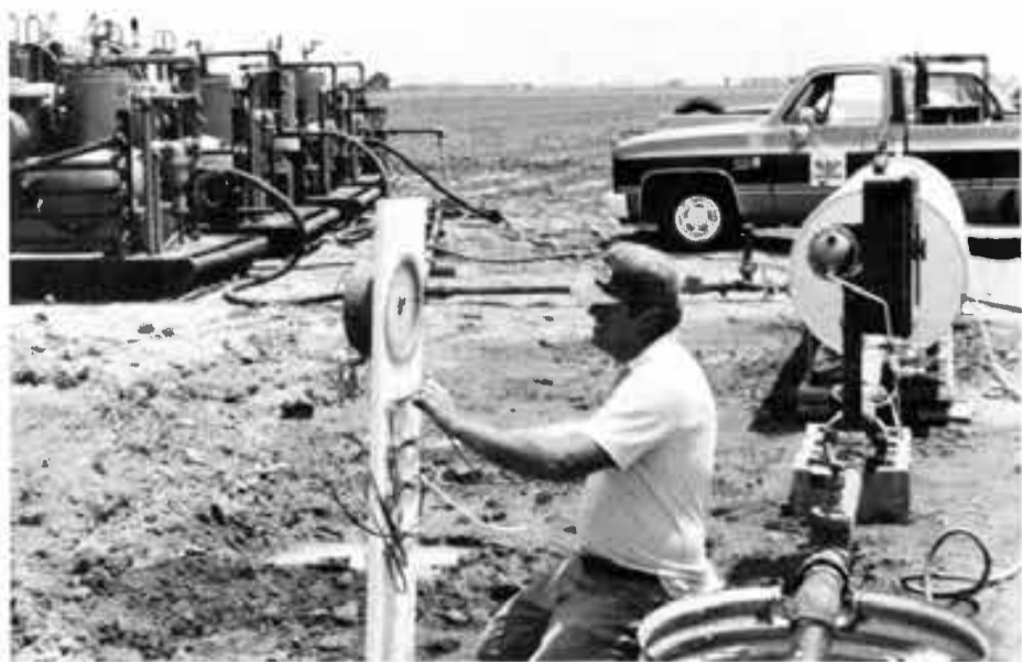
Idalou test site, air injection well (foreground), air monitoring equipment, and air compressors.
