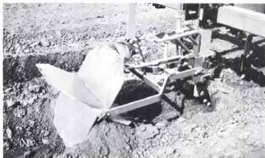
DAMMED FURROWS capture rainfall, hold moisture, stop runoff and prevent erosion.
