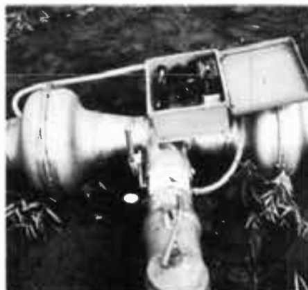
SURGE CONTROLLER box switches the water from one set to the other set on predetermined half-cycle times.
