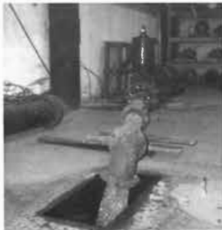
BREAK DOWN DARE —Goulds Pump Company performs a continuous tank test on one of their pumps to check performance and wear. This pump has been running for 700 hours.
