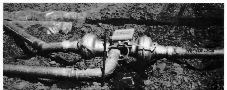
ONE VALVE of the surge system moves water to the low end of the field, while the other valve moves water to the top end. The ditch stop in the upper right hand corner divides the ditch into halves.
