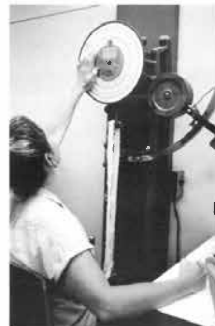
STRETCH —Testing the strength of cotton thread from open-end spinning machines determines the pounds of pressure required to break the thread.
