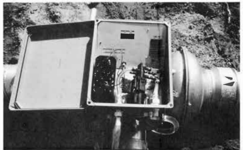
INTERNAL WORKINGS of a surge time control box shown close-up. Surge count shows the number of surges completed, time set is the length of each surge in hours and minutes and remaining time indicated is the time before the current surge is completed. These all help the irrigator manage his uniformity of application.
