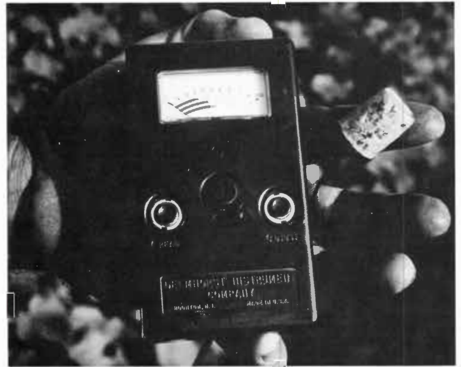
CONDUCTANCE METERS read electrical resistivity. The electrical resistivity indicates the percent moisture in the soil. The higher the meter reading, the greater the soil moisture.
