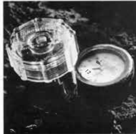
DRAWING MOISTURE from the surrounding soil, tensiometers show pressure gauge readings to help the irrigator determine his soil moisture.
