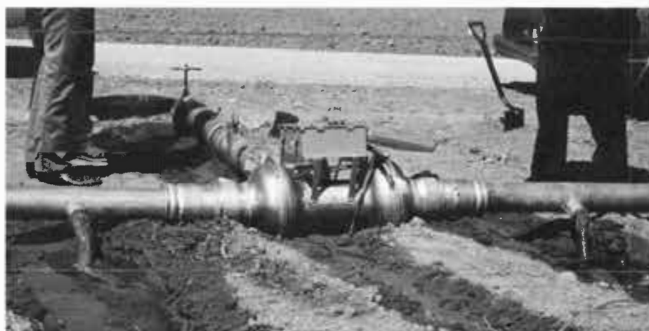
ANOTHER PERSPECTIVE of the surge valve shows the conclusion of one half-cycle time to the left as the second half-cycle time begins on the right.
