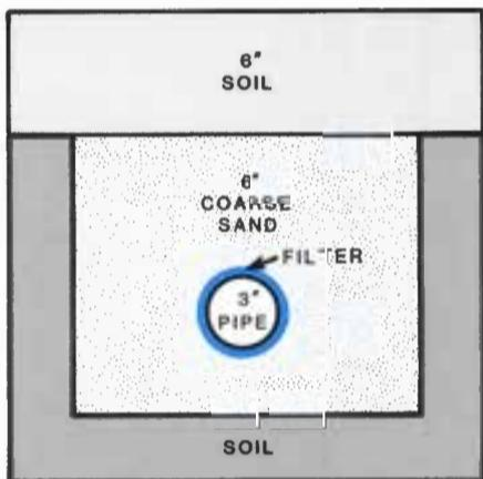
**FILTERS IN PLACE**—Sixteen-inch wide and 16-inch deep V-shaped trenches were dug in the base of the playa. A geotextile fabric filter was then slipped over three-inch diameter flexible plastic pipe like a sleeve. The fabric-covered pipe was then laid in a gravel bed in each trench, and six inches of sand and six inches of natural playa material backfilled each trench.
