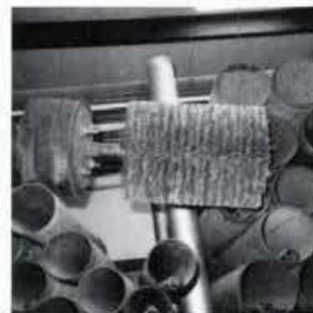
**JUST LIKE SCRUBBIN' A RUSTY BOLT—** The stiff nylon bristles of this street sweeper brush proved to be just what was needed to scrub out old well casings to remove the accumulated rust and scale deposits. Adding the brush to the bottom of the surge block has successfully rejuvenated several wells for the City of Lubbock.
