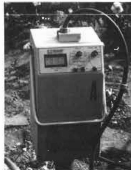
**PROBING FOR WATER**—A probe inside the neutron moisture meter is lowered down aluminum access tubes then neutron particles are emitted. The displayed figures translate to readings of soil moisture content.
