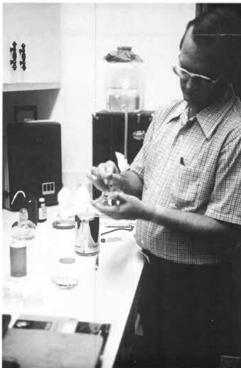
CONTAMINATED OR NOT? — Dan Seale, Engineer Technician in the High Plains Underground Water Conservation District No. 1 Field Support Section, conducts a fecal coliform test. The bacteria from the intestines of warm-blooded animals are a common source of water well contamination on the High Plains.
