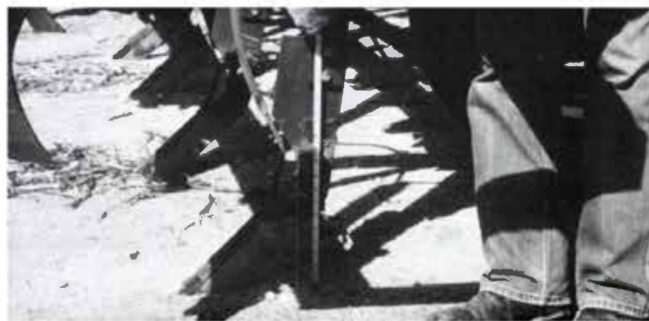
IT'S NOT AS DIFFICULT AS IT SEEMS — Max Lee wanted to prove to himself that it wouldn't be difficult to band phosphorus deep in the soil profile. So, in experiments to develop the right tool, he added six inches to the shank of a back-swept chisel. Thus far he has applied bands of phosphorus 13 inches deep in two plots of flat-tilled ground.
