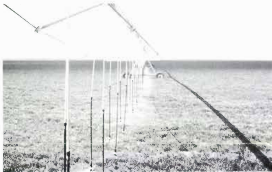
WATER RESOURCES SAVED — Troy Sublett of Hereford uses this LEPA system to help conserve water while irrigating wheat on his Deaf Smith County farm.
