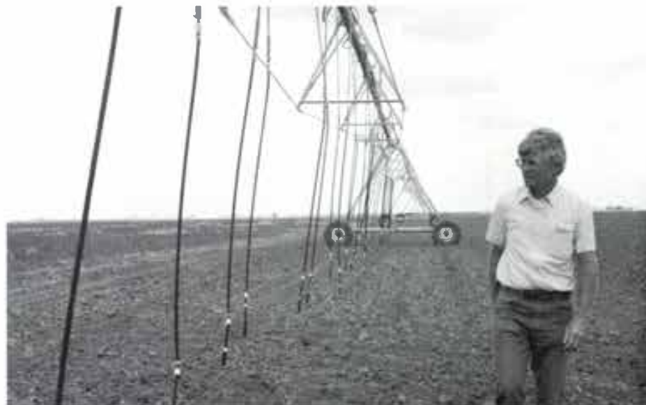
LOOKING OVER THE SYSTEM — Leon New, Texas Agricultural Extension Service Irrigation Specialist, examines a LEPA system equipped with Rainbird heads during the 1987 Randall County field demonstration day.
