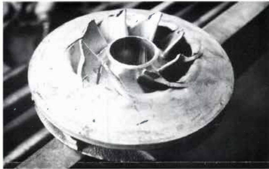
BUT IT WAS STILL PUMPING WATER — Worn-out or damaged pump parts, such as this impeller, will reduce pump performance and increase the monthly fuel cost to area producers. A careful watch of operating costs and periodic pump plant efficiency testing can signal a need for pump adjustments or repairs.
