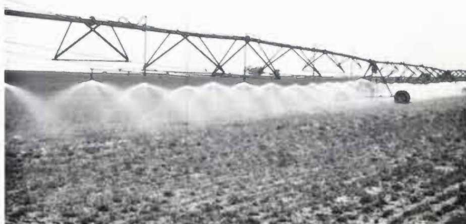
WATER SAVINGS — Conversion of center pivot systems from above line discharge to crop height discharge helps reduce water losses as much as 20 percent.
