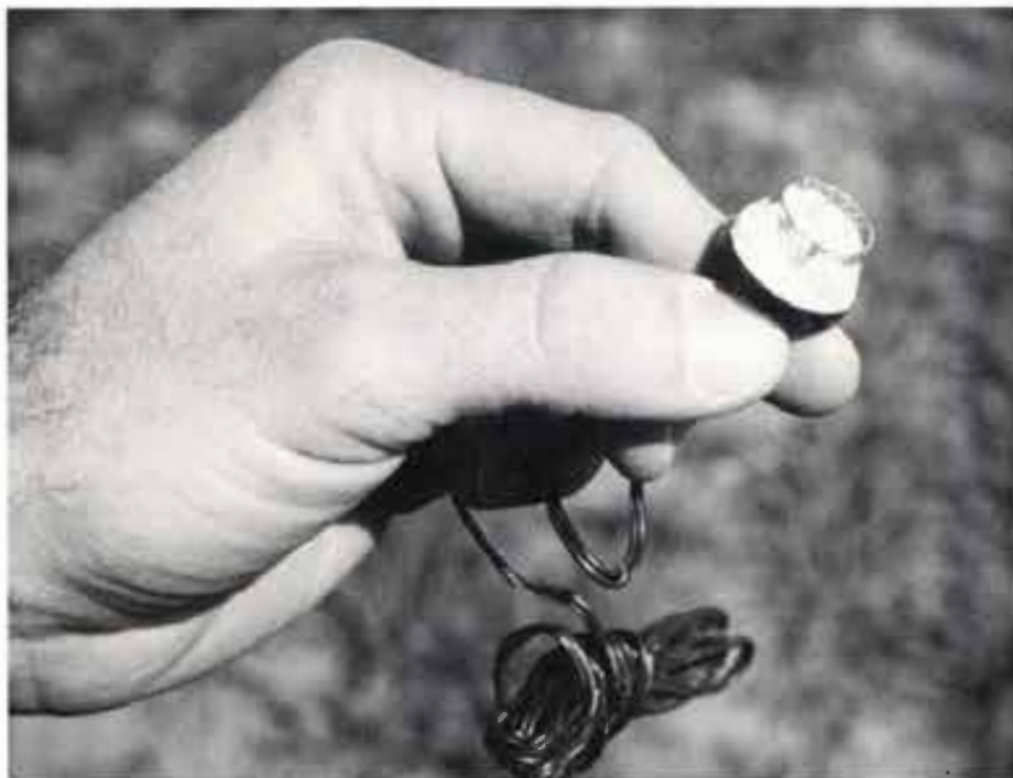
A WINDOW INTO THE SOIL — The gypsum has been scraped away to reveal the stainless steel electrodes that make up the core of a gypsum block. Electrical resistance between the electrodes registers on a resistance meter to measure soil moisture.
