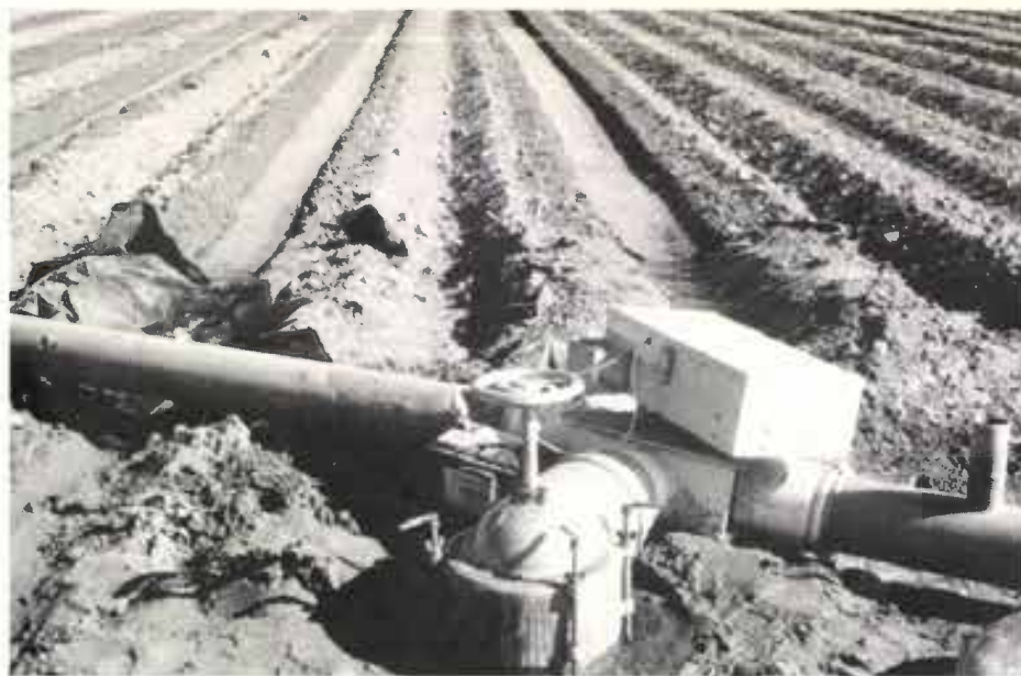
SURGE IRRIGATION IMPROVES WATER USE EFFICIENCIES —Ronald Schilling credits his surge valve (shown above) with a 15 percent increase in water use efficiency on his farm near Slaton.
