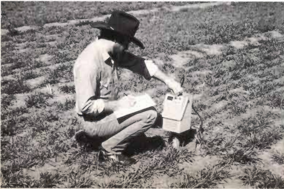
HOW DRY IS IT? — Agricultural Engineer Jerry Funck uses a neutron moisture meter to obtain soil moisture readings at one of the 250 soil moisture monitoring sites maintained by the High Plains Underground Water Conservation District No. 1.
