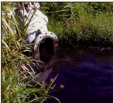
Sludge that the dredge pumps from the pond is sent through a pipe to a landfarm at Campbell Bayou.
