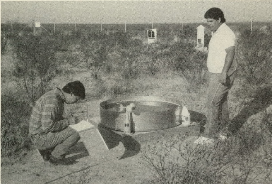
Julio Maldonado (l) and Joe Castro (r) record pan evaporation rates at the weather station located 10 miles northeast of Fort Hancock.
