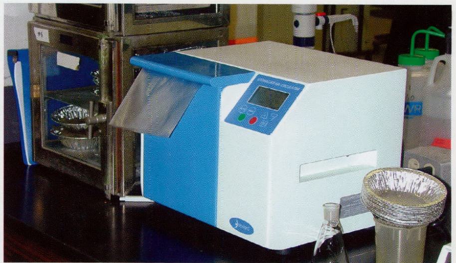
The stomacher is used to churn the compost with a buffer solution.
