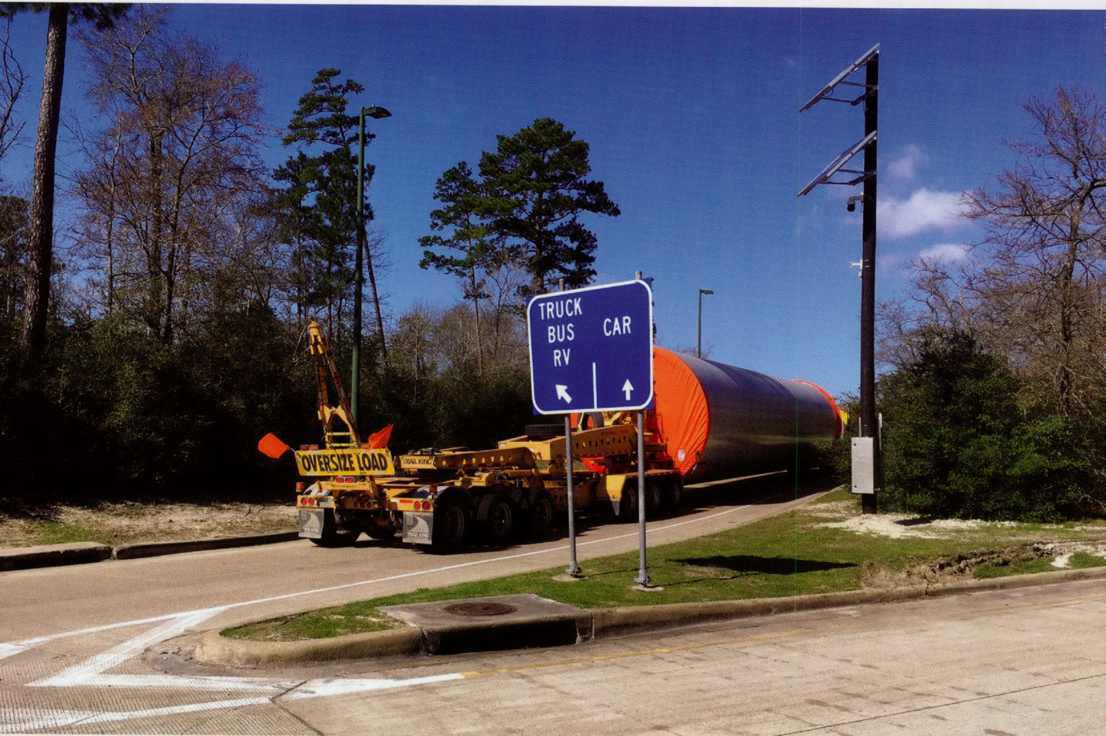
An oversized truck entering a northbound I-45 safety rest area. Notice the TTI-developed entry detection system located on the utility pole.
