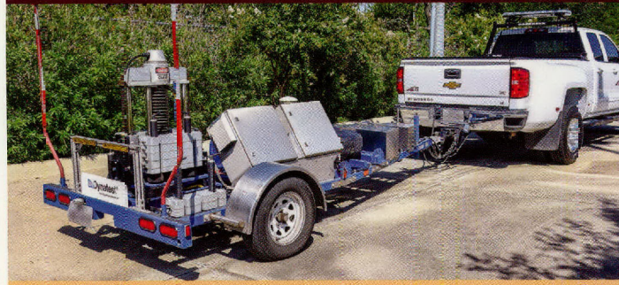
FWD is a nondestructive testing device widely used to evaluate pavement structural conditions.
