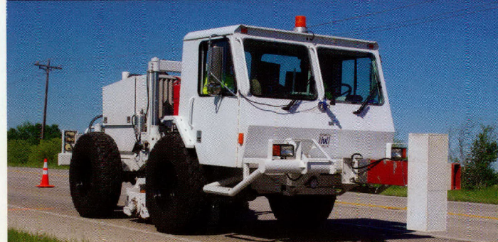
TPAD can nondestructively and nonintrusively measure pavement structural conditions.
