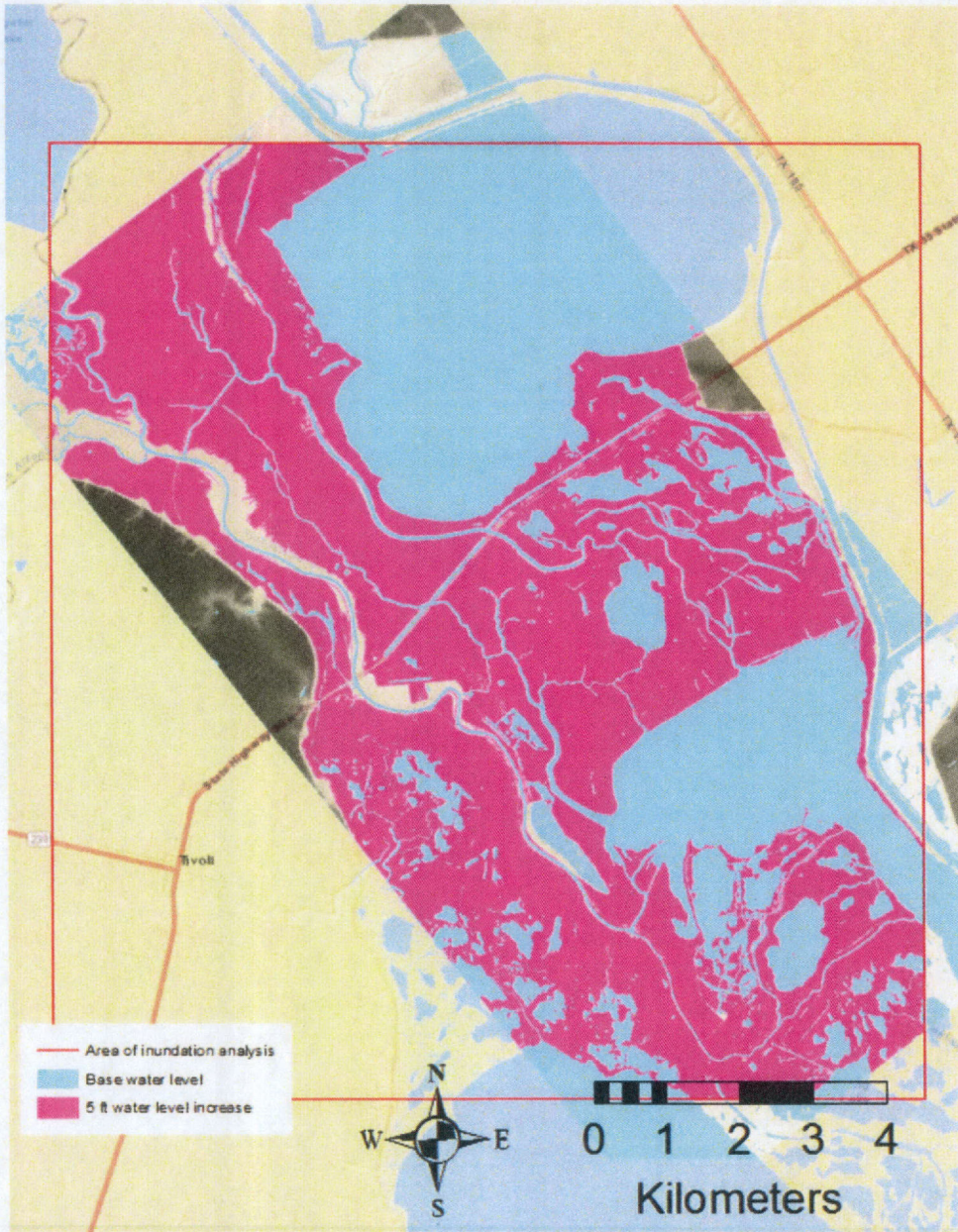
Figure B.7. Inundation resulting from a 5 ft Base water level increase
