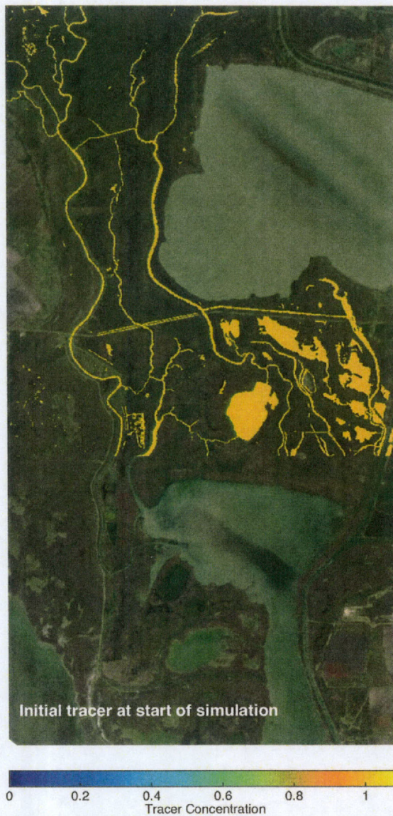
Figure D.1. Initial tracer distributed in the bayou and upstream sections of the Guadalupe River at the start of the simulation. Note that the colormap extends beyond the [0,1] range of tracer concentrations for better contrast with the satellite image.
