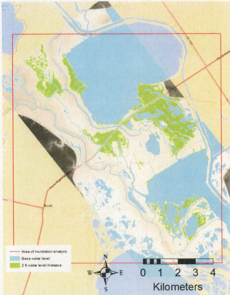
Figure B.4. Inundation resulting from a 2 ft Base water level increase
