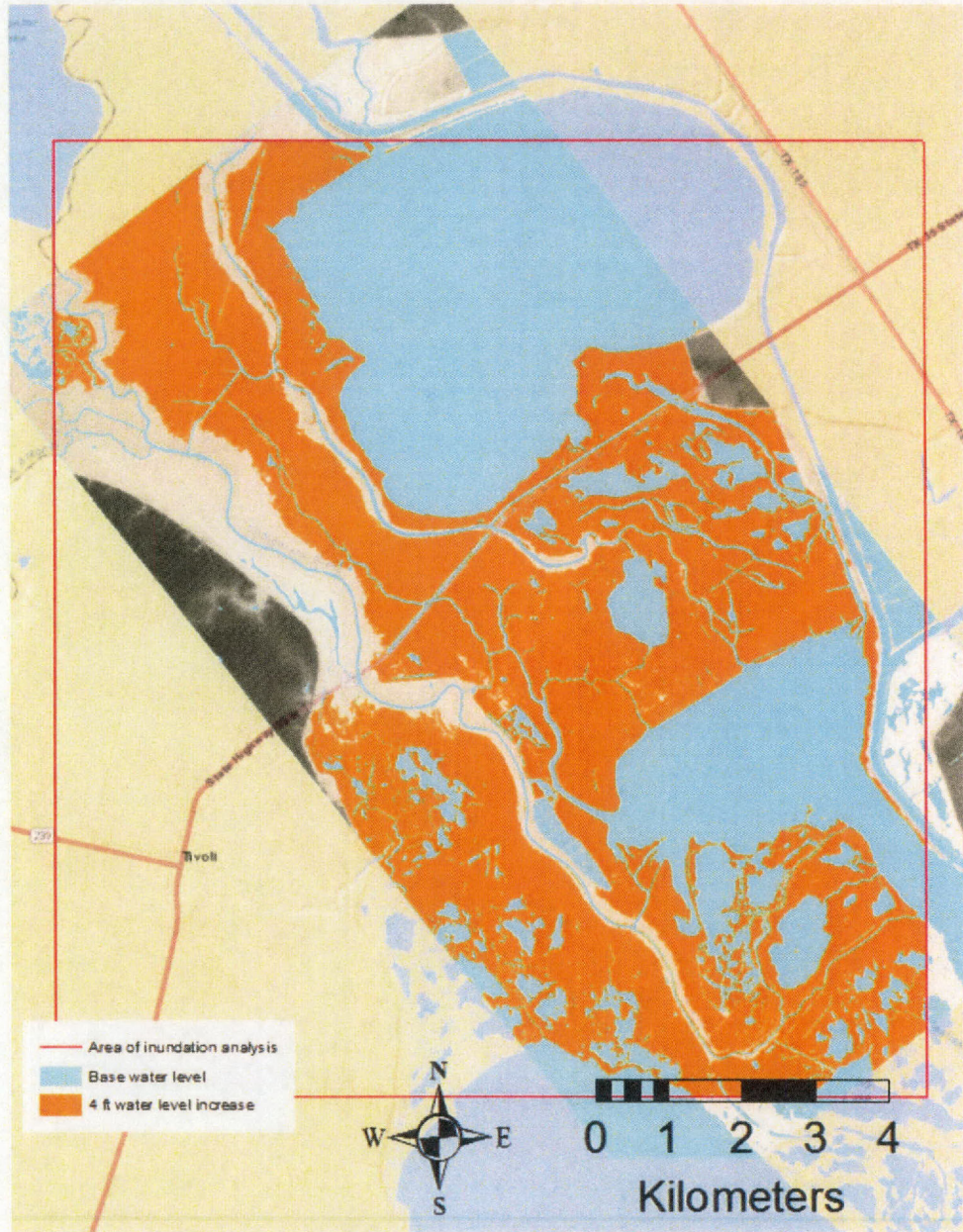
Figure B.6. Inundation resulting from a 4 ft Base water level increase
