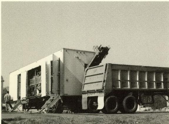
A new and improved Mobile Sludge Dewatering Unit became operational in 1984. The $250,000 unit incorporated aluminum and stainless steel to minimize rust and corrosion. Even industrial sludges can be dewatered by the upgraded unit.
