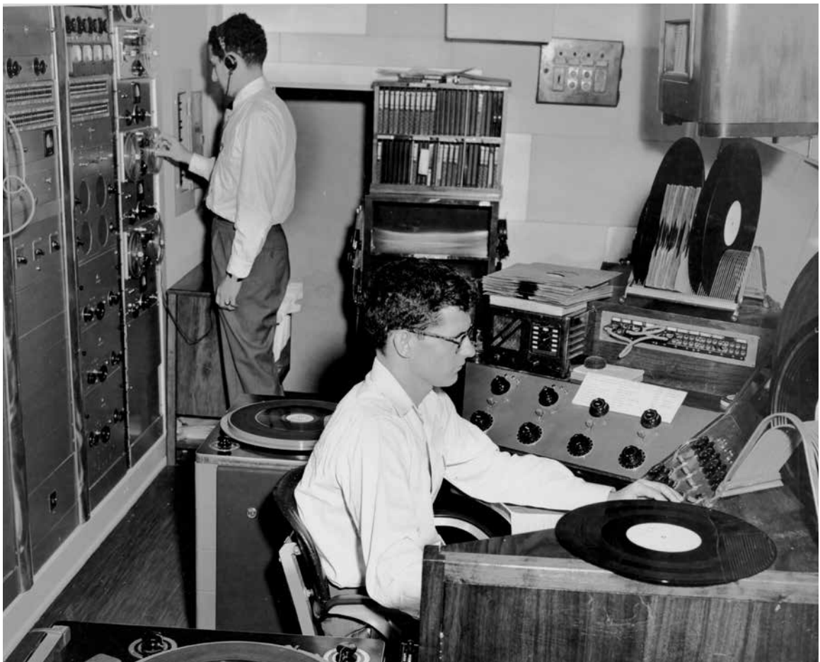
The large records shown in this undated studio interior photo are transcription discs, used for recording and replaying programs. Prior to magnetic recording tape, this was the most common method of recording and replaying radio programs
