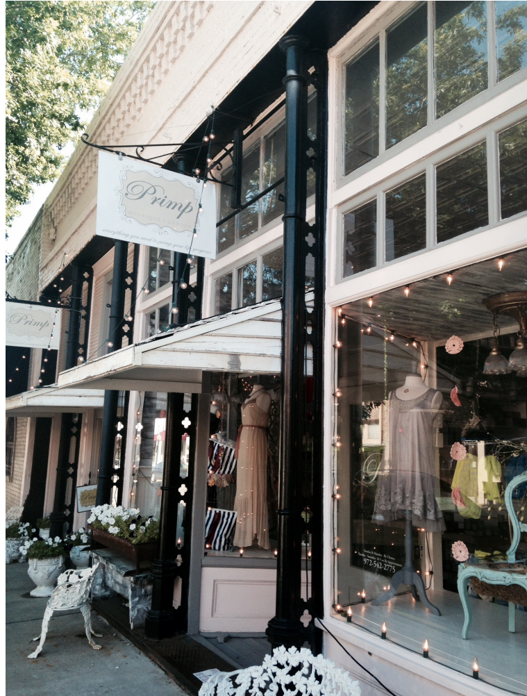
In form-based codes, shopfront requirements include a minimum percentage of transparent glass, primary entrances that open directly to the sidewalk, and specific standards for signs and awnings. These features are illustrated in this photo of Primp in McKinney's Main Street district.
