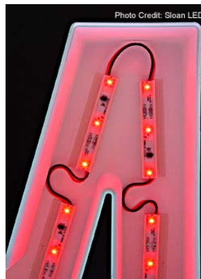
(Left) Letter LED lights lit. (Right) Neon in open face channel letter.
