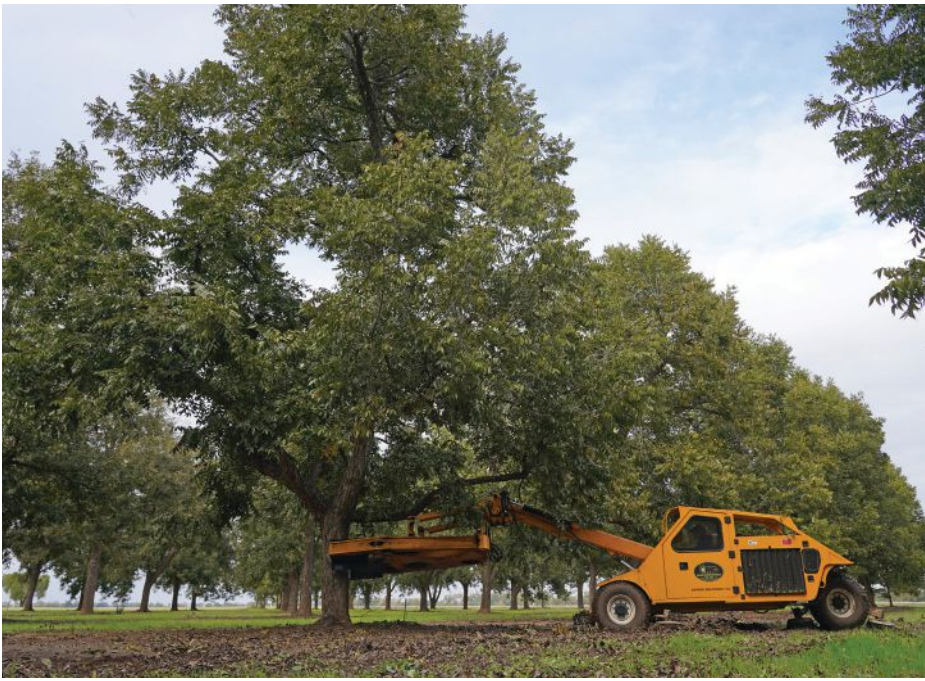
The machine shaker removes the pecans by shaking the tree. It's the first part in the harvest process.
