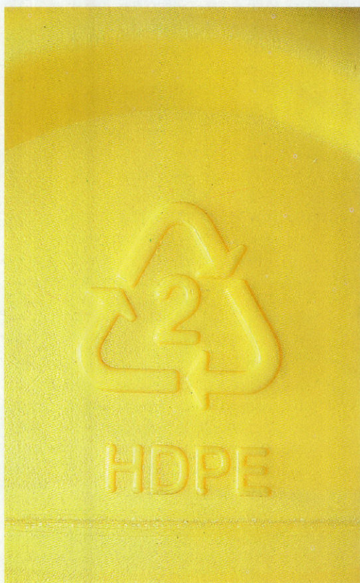
Last year, Texas became one of 16 states to require labeling of plastics. The triangular labels (above) contain numbers that tell plastic recyclers the type of plastic. Items such as plastic fittings (right) are shredded and shipped to industrial manufacturers.
