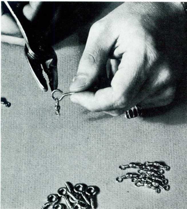
To make a jugfishing rig, begin by attaching a barrel swivel to a screw eye (left) and then liquid solder the eye into the top of an empty refrigerant can (right).
