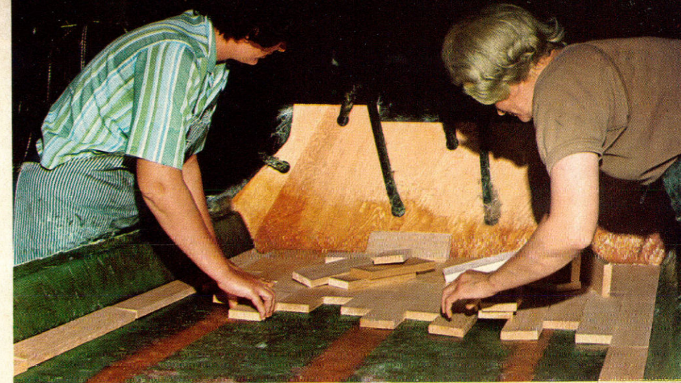
Balsa blocks used in hull provide extra safety flotation and rigidity.
