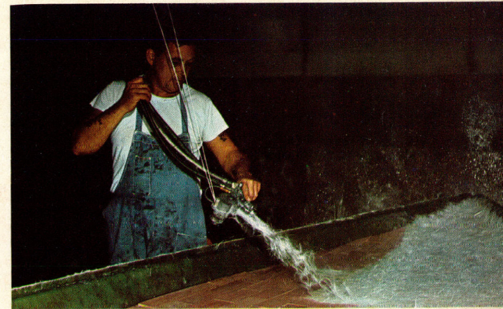
Durable seven-ply "lifeguard" fiberglass hull is protected with fire retardant coating.
