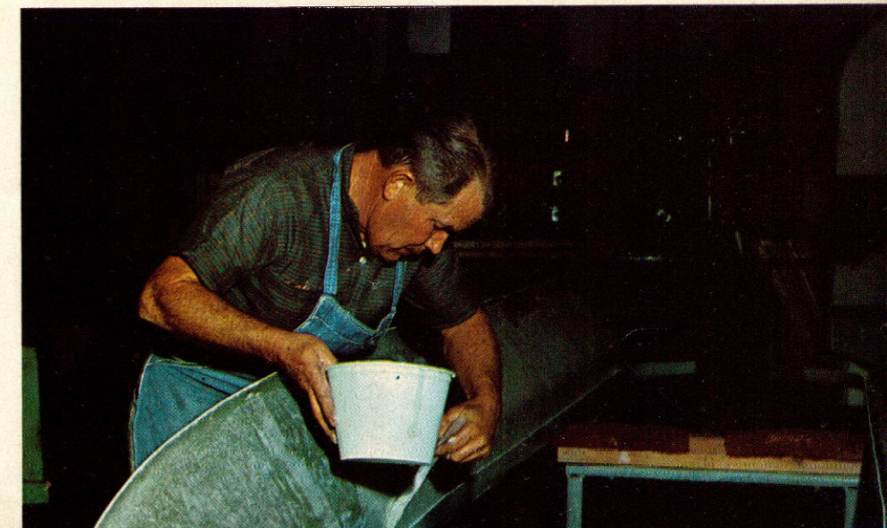
Durable seven-ply "lifeguard" fiberglass hull is protected with fire retardant coating.
