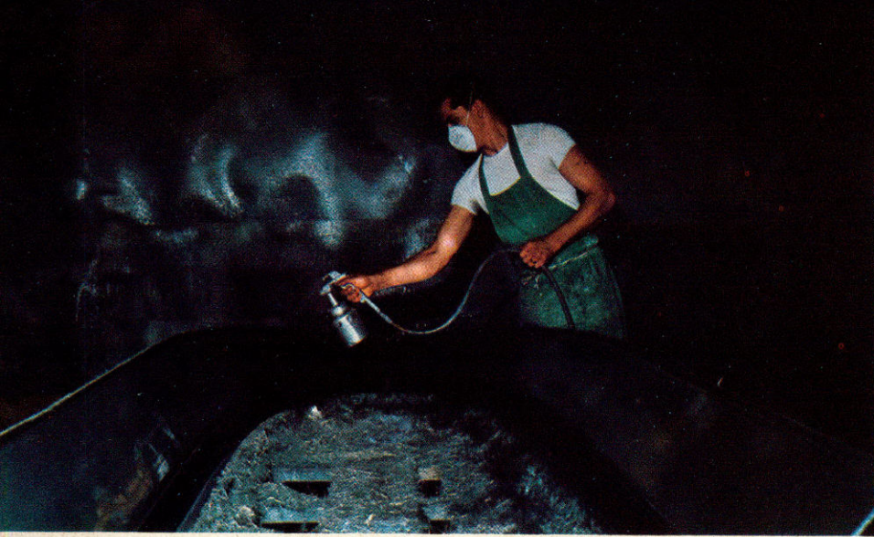
After permanent color coat, the two fiberglass halves are bonded together.
