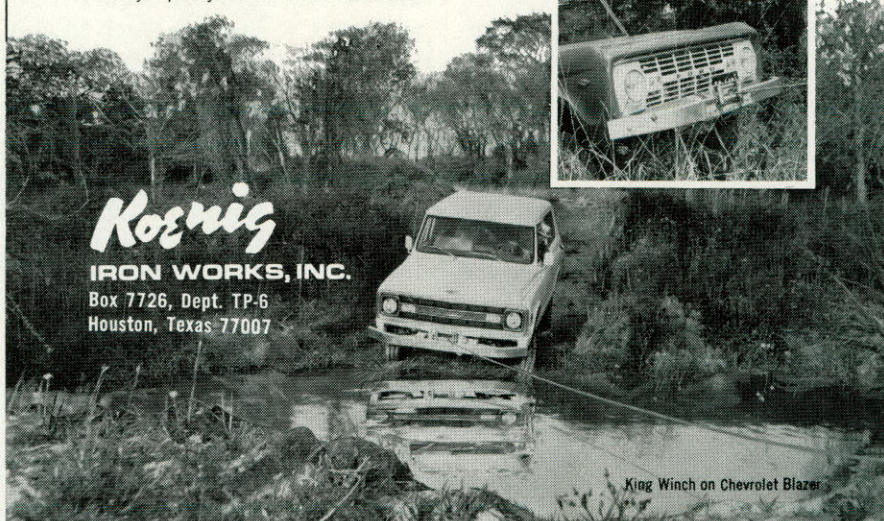
King Winch for Land-Rover, Bronco and other 4 WD vehicles has 8,000 lbs. pulling power.
