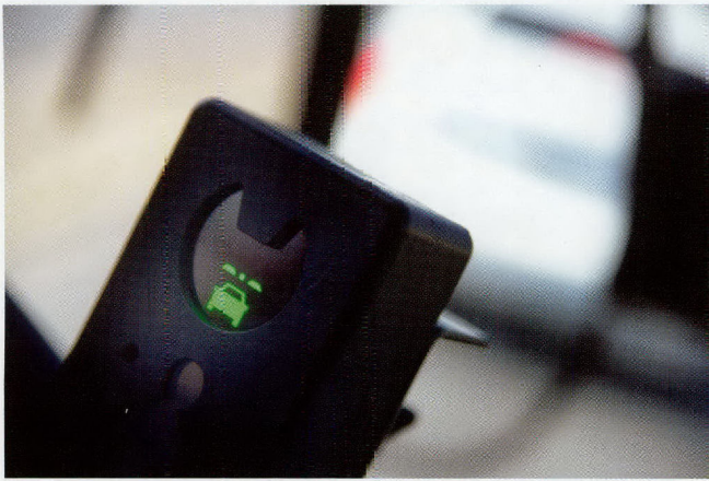
The MobileEye/Rosco Shield+™ collision-avoidance system has four different cameras that are essentially aimed at the blind spots on the bus and where pedestrians and bicyclists are most likely to show up and be in harm's way.
