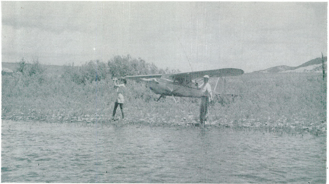
Shock absorbing qualities of Cessna's new patented safety landing gear, which is also resistant to normal ground looping, is a very desirable feature for one who wishes to bring his plane down for a rough landing beside a river or lake.
