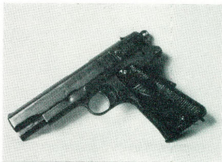
THE F. B. RADOM VIS MODEL 35. Weight: 29 ounces; over-all length: 7¾ inches; barrel length: 4¾ inches; magazine capacity: 8 cartridges; caliber: 9m/m Parabellum (Luger). The weapon is recoil operated—the barrel and breechblock being locked together at the instant of firing.
