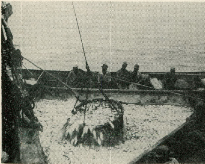
6. The menhaden then are transferred from the pocket of the seine to the hold of the mother ship by means of a brail net, which is raised and lowered by a power winch.
