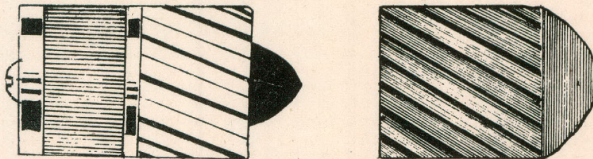
The original Model 1930 German Brenneke rifled shotgun slug, and (right) the American Nitro Express rifled slug—the ammunition maker's solution to the problem of firing a missile more accurately from a smoothbore arm.—Drawings by Wilson.
