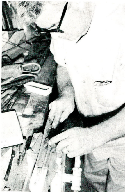
The groove is smoothed and finished before a thick layer of glass is plastered into it. As the barrel is inserted, the glass will be forced around the edges, cushioning the tube.
