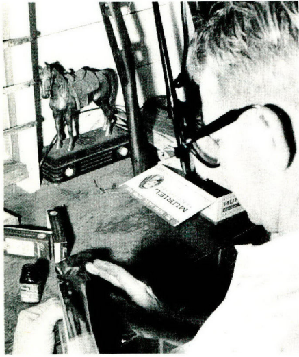
To finish the stock Stubby spreads on Tru-Oil with his fingers and smooths it out to a light finish. The stock takes on a smooth glamour.
