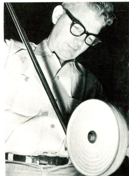
Stubby polishes the barrel, end to end, on a wheel coated with a special grinding compound.
