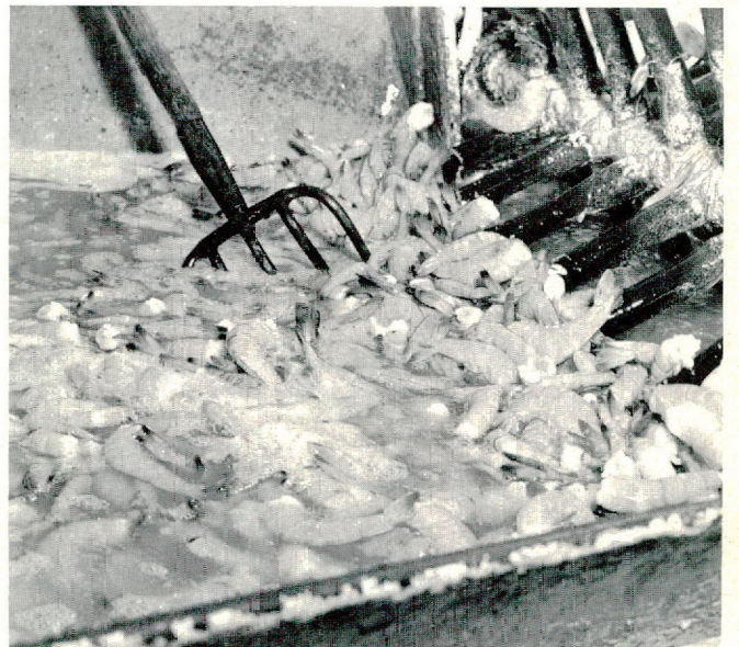
The motion of a spoked wheel sees to it that only a single layer of the shrimp is allowed to travel on the conveyor belt to the plant.
