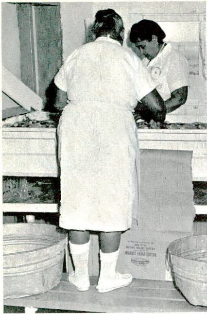
Broken and bad shrimp are removed by hand as they enter the plant. Sprays wash them as they move to the first of three grading machines.
