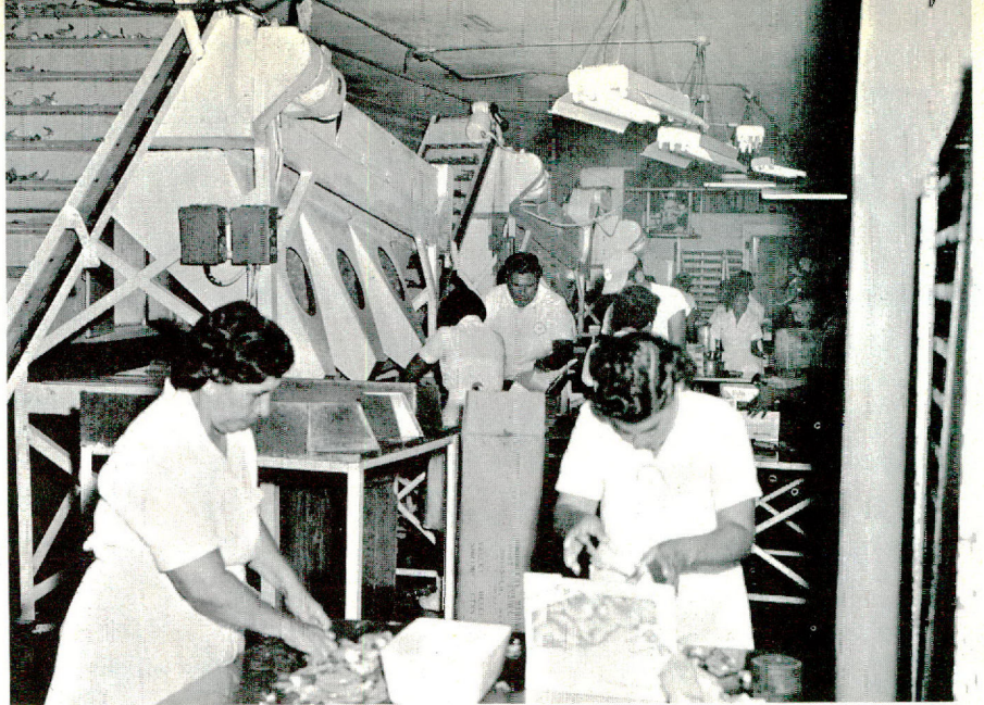
By machine-grading, first the smallest shrimp, then each slightly larger size, are picked out, only the largest reaching the last bin. Spot checks on uniformity are made for each grade.
