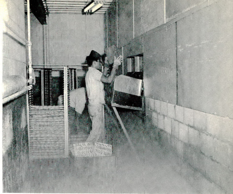
In next step, the frozen shrimp are emptied from the trays into a bin.
