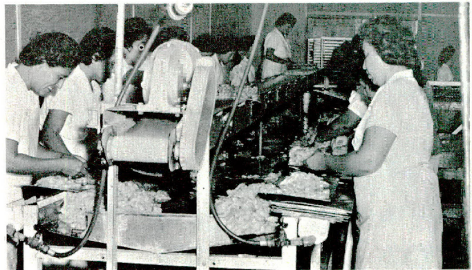
The shrimp, peeled, deveined and washed, are put on sterilized trays and sent to the quick-freezer.
