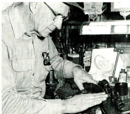
Coating the outside with grease is important.
