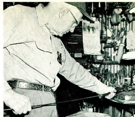
Dry patches, followed by Hoppes No. 9 and grease are parts of the Cline care procedure.
