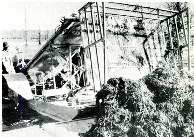
The load of vegetation is dumped onto a pair of waiting flat barges.
