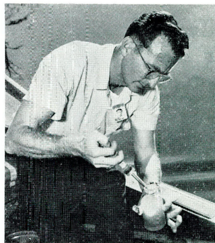
Debris and barnacles (left) must be regularly cleaned from diatom holder to prevent breakage of slides.
