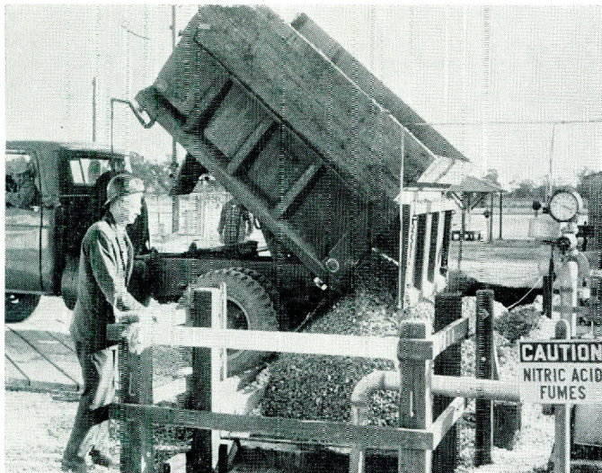
Alkaline, in the form of oyster shells (left), is used to neutralize acid content of industrial wastes.
