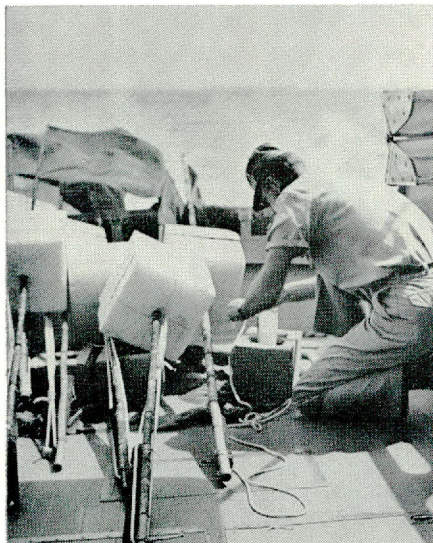
Concrete blocks are used for anchors.
